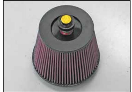
37. Install the filter minder along with the provided grommet into the K&N® air filter as shown.
