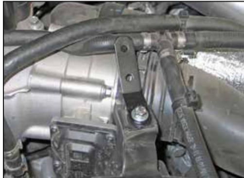
33. Install the coolant hose bracket onto the fan shroud as shown using the provided hardware.
