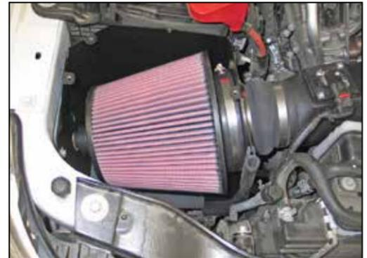
38. Feed the K&N® air filter top first into its location, then rotate it back and install onto the filter adapter. Secure the air filter with the provided hose clamp.
