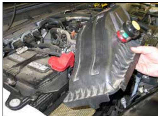
5. Remove the upper air box housing from the vehicle.
