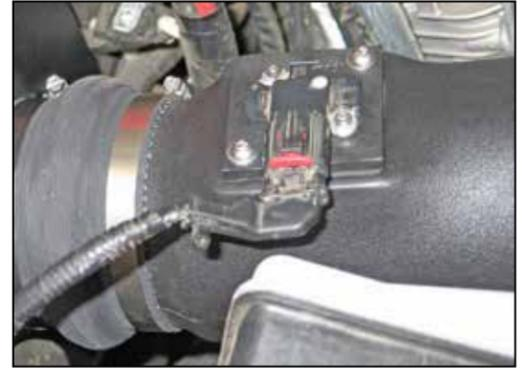
35. Reconnect the mass air sensor electrical connection. Secure the mass air sensor wiring harness to the A/C recharge pipe with the provided tie wrap.
