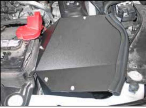
40. Attach the heat shield lid onto the heat shield and secure with the provided hardware.
