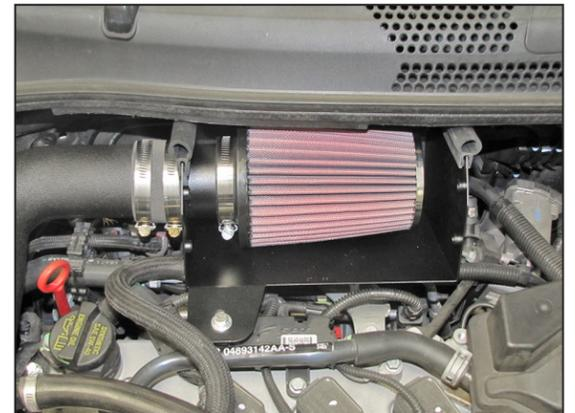
20. Install the K&N® air filter onto the heat shield tube and then secure with the provided hose clamp.
