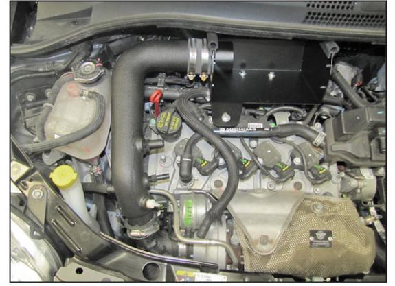
17. Install the K&N® intake tube into the factory turbo intake tube and then into the coupling hose on the heat shield tube. Secure the tube with the provided hose clamps.
