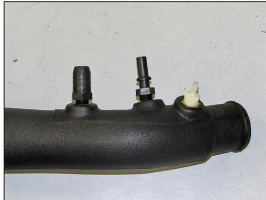
15. Install the three vent fittings into the K&N® intake tube as shown.
