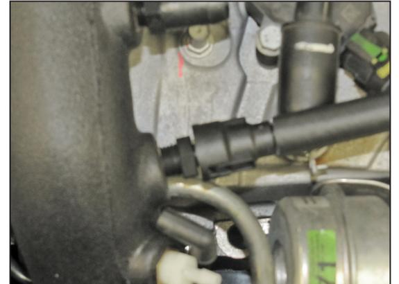
18. Connect the two vacuum lines to the fittings installed into the K&N® intake tube as shown.
