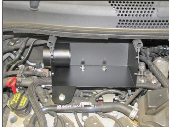
14. Install the heat shield onto the K&N® mounting bracket and the factory engine bracket and secure with the provided hardware.
