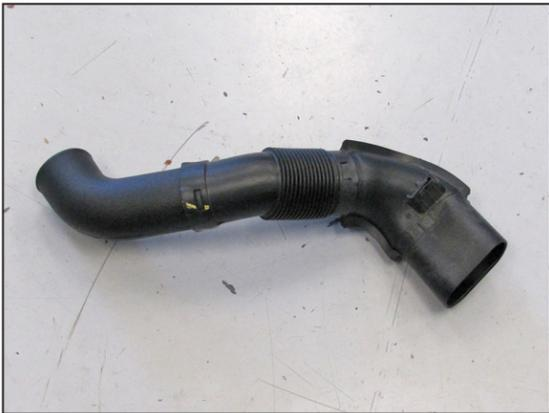
24. Install the K&N® fresh air intake tube into the factory fresh air duct as shown.
