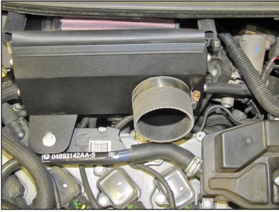
22. Install the remaining coupling hose (08727) onto the tube in the heat shield front cover and secure with the provided hose clamp.
