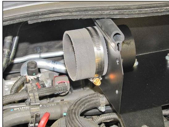
16. Install the coupling hose (08727) onto the heat shield tube as shown and secure with the provided hose clamp.
