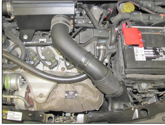
25. Install the fresh air assembly into the core support and then into the hose at the heat shield. Secure the assembly with the factory bolt and hose clamp provided.
