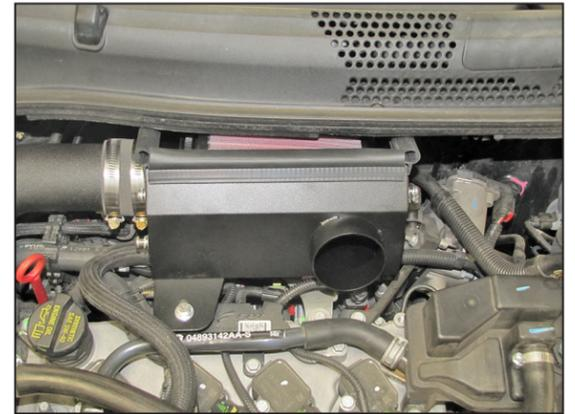
21. Install the heat shield cover and secure with the provided hardware.
