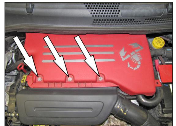
6. Loosen the three screws and remove the air filter housing lid and air filter.
