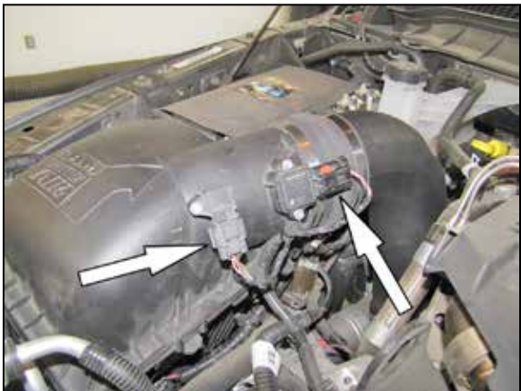
12. Reconnect the mass air sensor and temperature sensor electrical connections.
