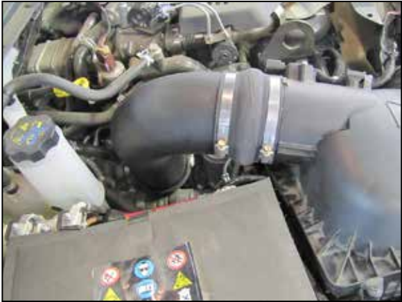
11. Install K&N® intake tube into the factory turbo inlet hose and then into coupling hose (08695). Secure K&N® intake tube with provided hose clamps.
