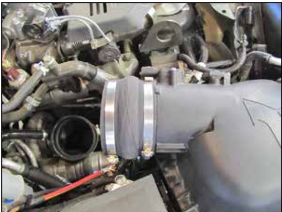
10. Install coupling hose (08695) onto air box assembly. Secure with provided hose clamp.
