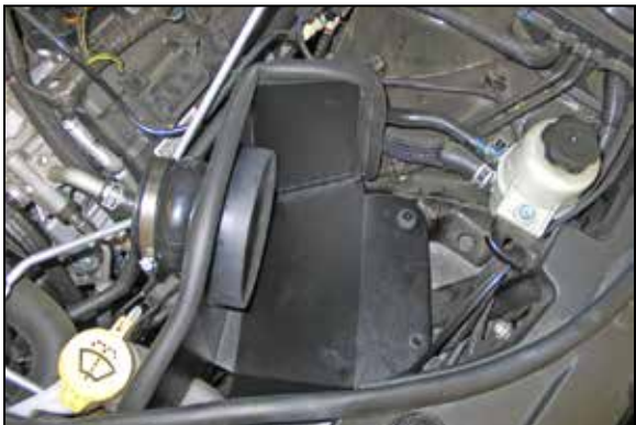
15. Set the heat shield into the vehicle so that the mounting grommets slide over the factory airbox mounting studs.
