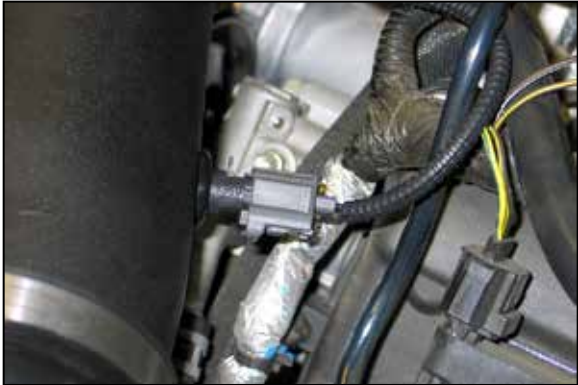
24. Connect the inlet air temperature sensor extension harness into the factory electrical connection and then connect the other end into the inlet air temperature sensor as shown. NOTE: There are two different types of sensors, be sure to choose the correct harness extension for the sensor used.
