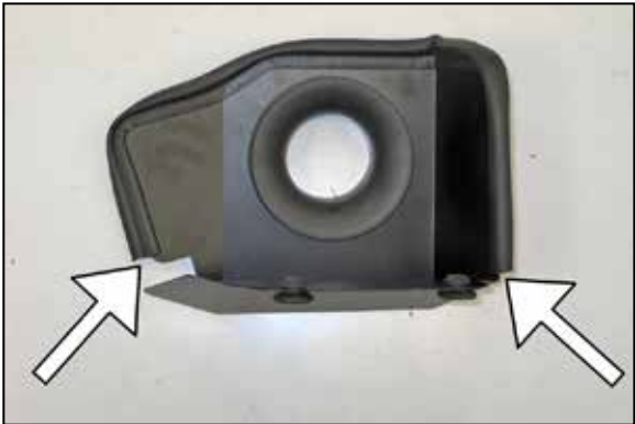
13. Install the provided edge trim onto the heat shield as shown. NOTE: Some trimming of the edge trim will be necessary.
