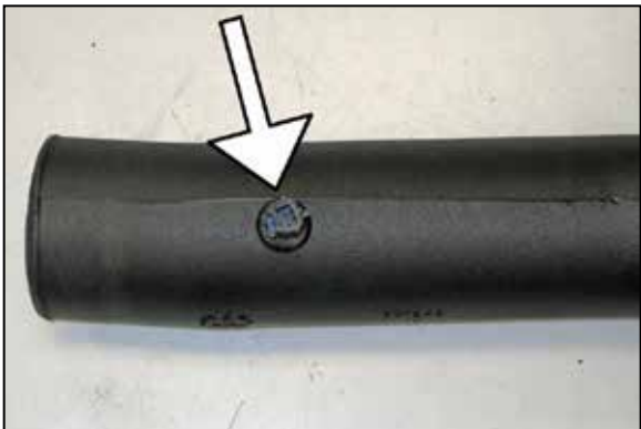
20. Install the inlet air temperature sensor into the K&N® intake tube. NOTE: Be sure to remove the O-ring from the inlet air temperature sensor before installing.
