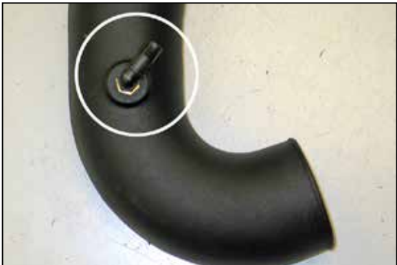
21. Install the 90° npt fitting into the K&N® intake tube as shown. NOTE: Plastic NPT fittings are easy to cross thread. Install the vent fitting “hand” tight, then turn it two complete turns with a wrench.
