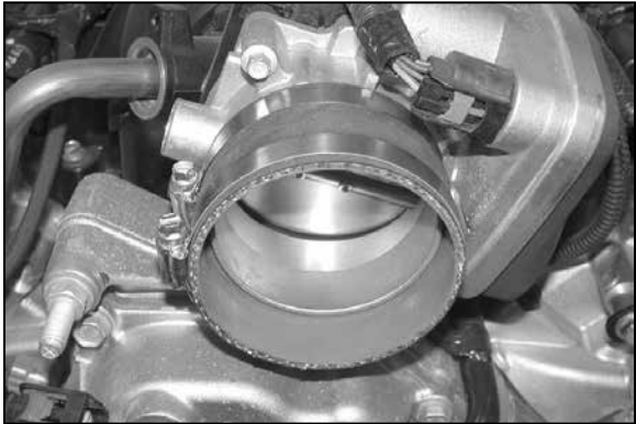
17. Install the provided silicone hose (08630) onto the throttle body and secure with the provided hose clamp.
