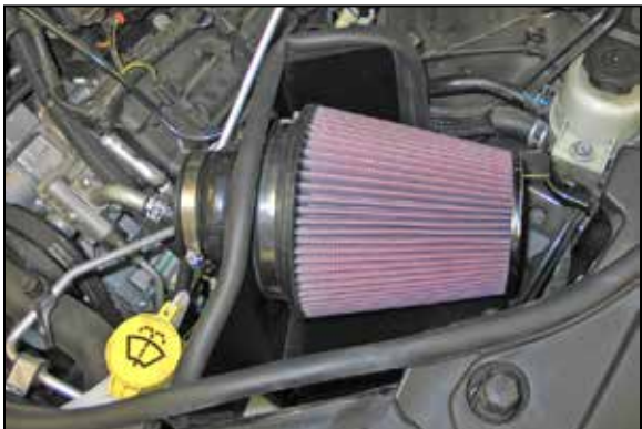
16. Install the K&N® filter onto the adapter and secure with the provided hose clamp. NOTE: Drycharger® air filter wrap; part # RF-1041DK is available to purchase separately. To learn more about Drycharger® filter wraps or look up color availability please visit http://www.knfilters.com ®.
