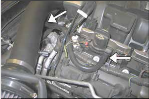
23. Install the crankcase vent hose onto the 90° vent fitting and then attach the open end to the valve cover port.
