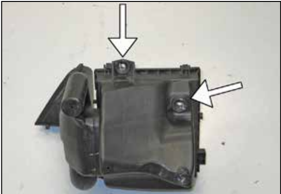
11. Remove two of the factory airbox mounting grommets from the lower airbox.
