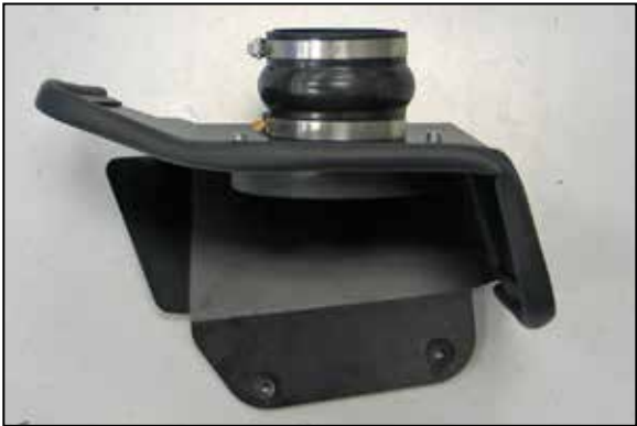
14. Install the provided silicone hump hose (084057) onto the filter adapter and secure with the provided hose clamp.
