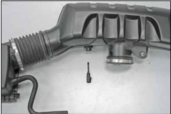
18. Release the locking tab and the remove the inlet air temperature sensor from the factory intake tube by twisting counter clockwise. NOTE: The inlet air temperature sensor is very fragile; take care to avoid damage while handling the sensor.
