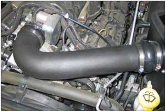
21. Install the K&N® intake tube into the hump hose at the filter adapter and then into the hose at the throttle body. Adjust the tube and heat shield for best fit and clearance and then secure with the provided hose clamps
