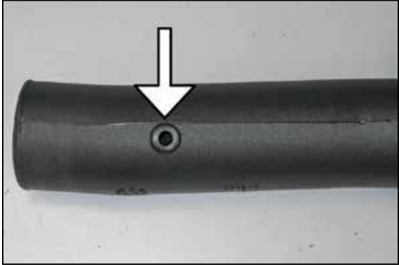
19. Install the provided grommet into the K&N® intake tube as shown.
