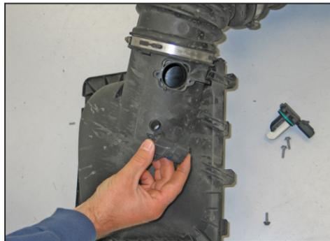
17. Remove the screws securing the mass air sensor and temperature sensor to the air box.
