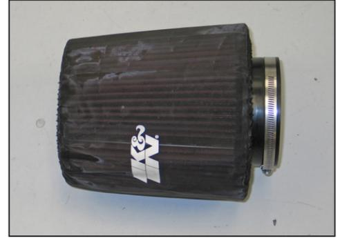
19. If the vehicle is going to be operated in extreme wet or snow conditions, it is recommended that a Drycharger air filter wrap, sold separately, be installed onto the K&N air filter.
