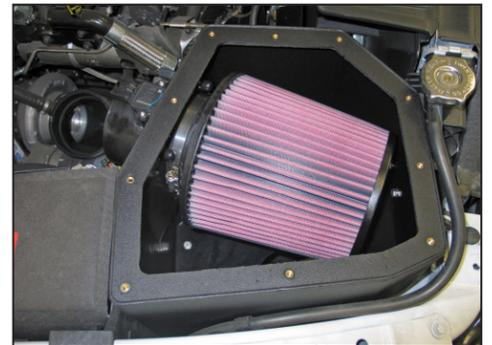
21. Install the K&N mass air housing onto the mounting studs and into the K&N air filter inlet. Secure the housing to the studs with the provided hardware and then secure the air filter with the provided hose clamp.
