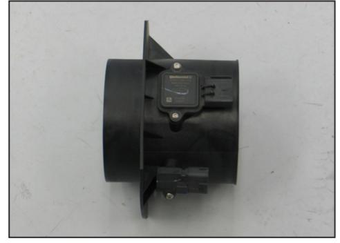
18. Install the mass air sensor and temperature sensor into the K&N mass air sensor housing using a twisting motion to aid installation; secure with the provided hardware.
