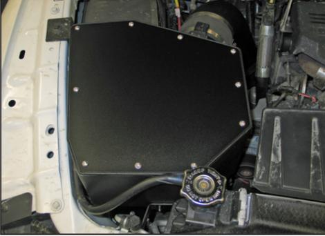
24. Install the air box lid and secure with the provided hardware.
