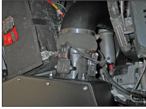
25. Reconnect the mass air sensor and temperature sensor electrical connections.
