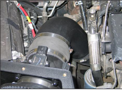
23. Install the K&N® intake tube into the factory turbo inlet hose and then connect the K&N® hose to the K&N® mass air sensor housing. Secure the intake tube with the hose clamps provided.
