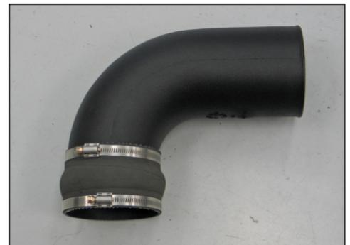
22. Install the provided silicone hose (08695) and hose clamps onto the K&N intake tube as shown. **NOTE: Do not completely tighten at this time.**
