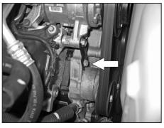
21a. On 2008 and later model year vehicles, remove the lower A/C bracket mounting bolt shown.
