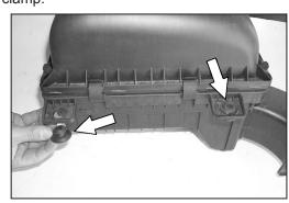
9. Remove the two rubber bushings from the factory air box as shown.
