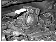
8a. Install the provided silicone hose (08051) onto the throttle body and secure with the provided hose clamp.
