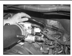
30e. Reinstall the vent tube assembly into the rubber fittings in each valve cover so that the "T" fitting is now on the drivers side of the engine facing forward.
