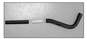
30g. On 2008 and later model year vehicles, insert the provided hose mender into the remaining piece of the factor vent hose and then cut the provided vent hose to 5" length connect onto the hose mender.
