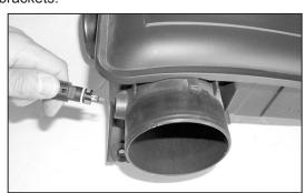
23. On models that come equipped with temp sensors, remove the air temp sensor from the resonator box as shown.
