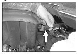
7. On 2002-2007 model year vehicles, disconnect the crank case vent hose from resonator box as shown. Then remove resonator box from vehicle.
