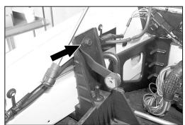
18a. Install the twisted "L" bracket with the bolt that was removed in step 18. Do not tighten bolt completely.
