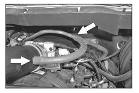
31. Connect the provided vent hose onto the "T" fitting then connect the other end onto the intake tube.
