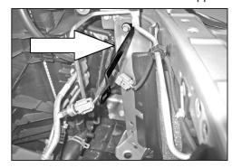
17a. On 2009 and later model vehicles, install the provided heat shield mounting bracket onto the radiator core support using the bolt removed in the previous step.
