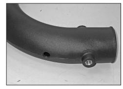
24. On models that come equipped with temp sensors, drill a 7/8" hole in the K&N® intake tube at the drill point.
