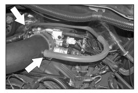
32. On models with the crank case vent tube connected to the passenger side valve cover, connect the provided silicone hose onto the factory vent tube and then route the crank case tube assembly behind the throttle body as shown and connect the open end onto the K&N® intake tube.
