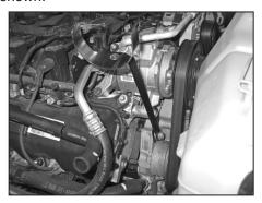
21b. On 2008 and later model year vehicles, install the tube mounting bracket using the bolt removed in the previous step and the spacer provided.
