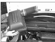
3. Lift up firmly to release the air box from mounting studs, then remove completely.
