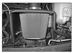
34. Install the K&N® air filter onto the intake tube as shown.
