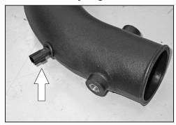
27. Install the air temp sensor into the  $K\&N^{\mbox{\scriptsize 0}}$  intake tube as shown.
