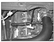
33. On 2008 and later model year vehicles, connect the crank case vent hose assembly to the valve cover port and intake tube vent fitting as shown.
