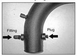
27a. On 2002-2007 model year vehicles, install the NPT fitting and NPT plug as shown.
