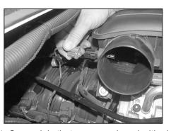
4. On models that come equipped with air temp sensors, unplug the air temp. sensor electrical connection as shown.
