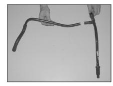
30c. Cut the crank case vent tube 1" from the "T" fitting as shown.
