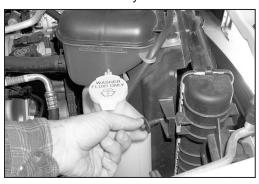
15. On 2008 & earlier vehicles, remove the 13mm bolt from the upper fan shroud as shown.
