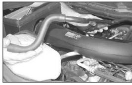
30a. On models that the crank case vent hose is connected to the "T" on the passengers side of the engine, remove the complete vent tube assembly from the rubber fittings in each valve cover as shown.
