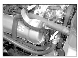
21. On 2002-2007 model year vehicles, install the saddle bracket assembly with the stud that was removed in step 20.
