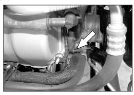
20. On 2002-2007 model year vehicles, use a 8mm socket, remove the stud that retains the oil fill bracket.
