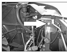
17. On 2009 and later model vehicles, remove the bolt shown from the radiator core support.
