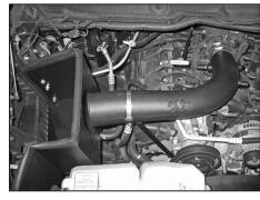
28. Install the K&N® intake tube into the silicone hose at the throttle body and align to the mounting bracket, secure the intake tube with the hose clamps provided.
