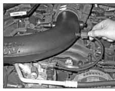
29. On models equipped with an air temperature sensor, connect the harness extension into the factory connector and then connect the open end onto the air temperature sensor.
