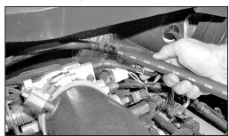
30. On models that the crank case vent hose is connected to the "T" on the drivers side of the engine, remove the factory vent hose from the "T" fitting as shown.
