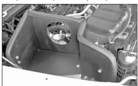
22. Install the heat shield onto the factory air box studs then mount to the previously installed brackets.
