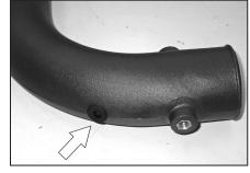
25. Install the provided grommet into the K&N® intake tube as shown.
