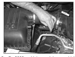
2a. On 2008 and later model year vehicles, disconnect the crank case vent hose from the air box as shown.
