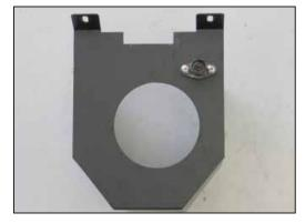
18. Install the inlet air temperature sensor into the heat shield as shown and secure with the provided hardware.
