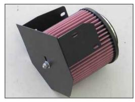
19. Attach the heat shield back plate to the K&N® filter as shown and secure with the provided hardware.
