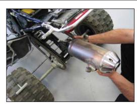
6. Remove the two bolts which secure the muffler to the chassis and then remove the muffler assembly from the vehicle.
