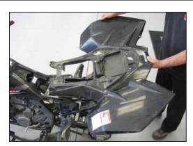
4. Remove the rear body work from the vehicle.
