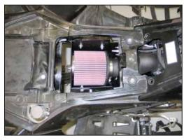
27. Tighten the hose clamps that secure the intake tube to the throttle body and air filter. Align the heat shield and tighten all of the mounting hardware.
