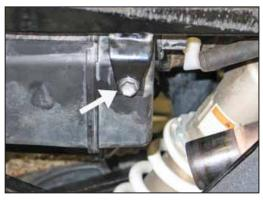
10. Remove the two bolts which secure the air box to the frame.
