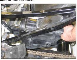
11. Remove the air box assembly from the vehicle by sliding it forward and then pulling trough the bottom of the chassis.
