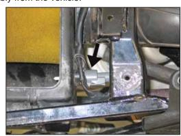
7. Disconnect the inlet air temperature sensor electrical connection.
