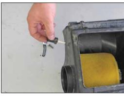
17. Remove the screws securing the inlet air temperature sensor and then remove the sensor from the factory air box.
