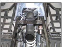
15. Install the intake tube into the silicone hose at the throttle body and secure with the provided hose clamp. Do not completely tighten at this time.
