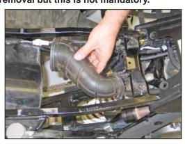
12. Loosen the hose clamp which secures the intake tube to the throttle body. Remove the intake tube from the vehicle.
