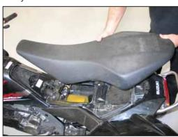
2. Release the seat latch and then remove the seat from the vehicle.
