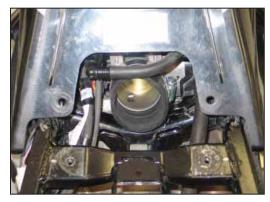
13. Install the provided silicone hose onto the throttle body and secure with the provided hose clamp.
