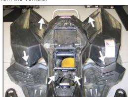
3. Remove the six bolts which secure the rear body work to the vehicle.
