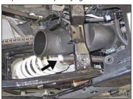
16. Insert the crank case vent fitting into the grommet installed into the intake tube as shown.
