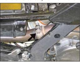
5. Loosen the clamp which secures the muffler inlet to the exhaust pipe.
