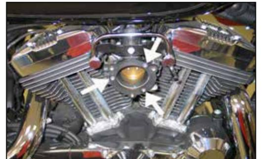
8. Install the K&N<sup>®</sup> intake tube adapter onto the throttle body using the provided hardware.
