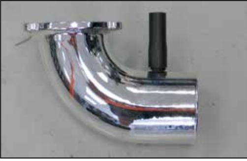
9. Cut the provided crankcase vent hose to a length of 1.75" and install onto the K&N® intake tube as shown.
