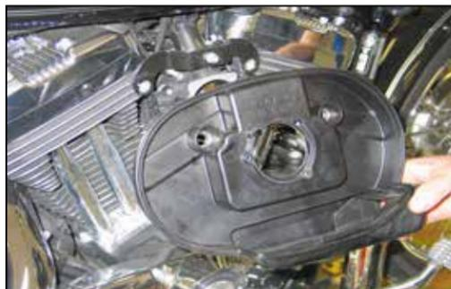
6. Remove the air filter base as shown.
