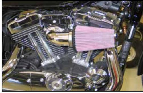
11. Install the K&N® air filter onto the K&N® intake tube and secure with the provided hose clamp. A black hose clamp is being supplied with kit. This clamp is intended to clamp the filter to the intake tube.
