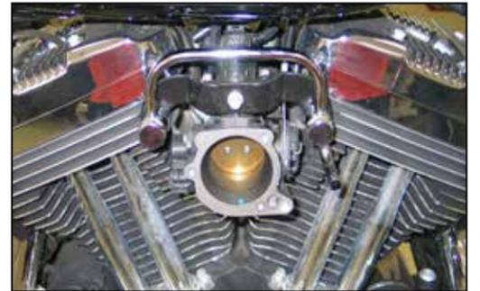
7. Install the K&N<sup>®</sup> crankcase breather tube onto the vehicle using the provided hardware.
