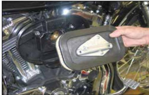
4. Remove the air filter as shown.
