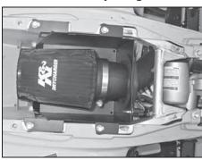
20. Install the K&N® air filter assembly onto the intake tube and secure with the provided hose clamp
