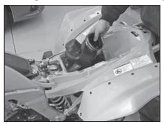
12. Remove the intake resonator from the vehicle
