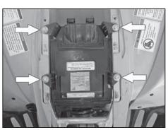
8. Remove the four bolts securing the air box to the frame.
