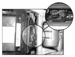
6. Remove the screw which secures the inlet air temperature sensor to the air box. Then remove the air temperature sensor from the air box.
