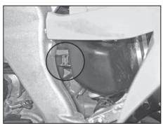
10. Release the spring clamp securing the crank case vent line to the intake resonator chamber and then disconnect the crank case vent line.
