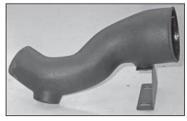
16. Install the provided tube mounting bracket (070120) onto the K&N® intake tube and secure with the provided hardware.
