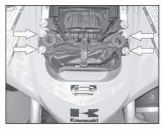
Remove the four bolts which secure the tool tray.
