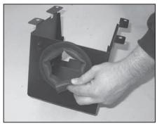
13. Install the provided edge trim into the heat shield as shown.
