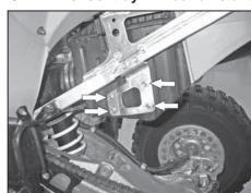
4. Remove the eight bolts which secure the factory air box to the frame side mounts, there are four bolts on the left side and four bolts on the right side of the air box.
