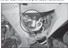
18. Install the 90° vent fitting into the K&N® intake tube as shown. Then connect the factory crank case vent hose to the fitting and secure with the factory clamp.
