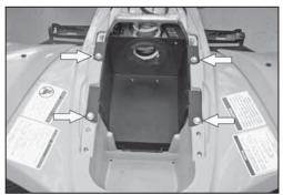
14. Install the K&N® air box into the chassis and secure with the factory air box mounting bolts. NOTE: Due to manufacturing tolerances, the air box may be a tight fit passing through the frame rails.
