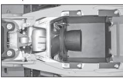
17. Install the K&N® intake tube through the heat shield into position. Be patient and take your time, it is a tight fit but it will fit. It may be helpful to loosen the heat shield while installing the intake tube. Secure the intake tube to the factory intake hose with the factory clamp. Secure the tube bracket to the air box with the provided hardware.
