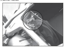
15. Install the air temperature sensor into the heat shield and secure with the provided hardware.
