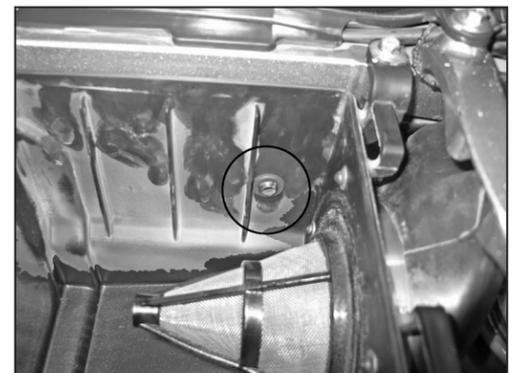
7. Push the crank case vent fitting and grommet out of the air box from the inside out to remove it from the air box.
