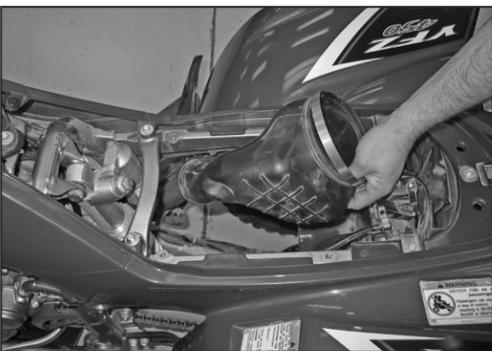
12. Remove the intake tube from the vehicle as shown.
