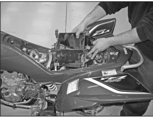
10. Remove the air box from the vehicle as shown. **NOTE: K&N Engineering, Inc., recommends that customers do not discard factory air intake.**
