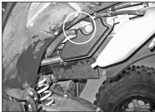
4. Release the spring clamp which secures the crank case breather hose to the chamber. Then disconnect the crank case vent hose.
