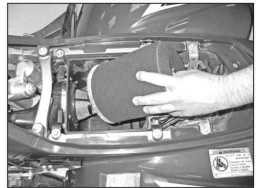
6. Loosen the air filter retaining bolt and then remove the stock air filter from the air box.
