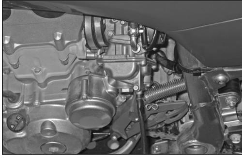
13. Disconnect the crank case vent hose from the vent fitting. Loosen the hose clamp which secures the carburetor to manifold hose; disconnect the carburetor from the manifold and pull it out to the side of the chassis as shown.
