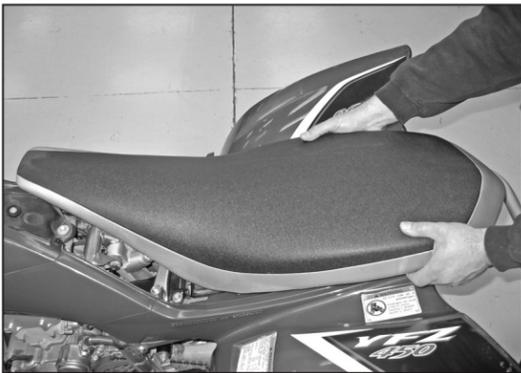
2. Release and remove the seat from the vehicle as shown.
