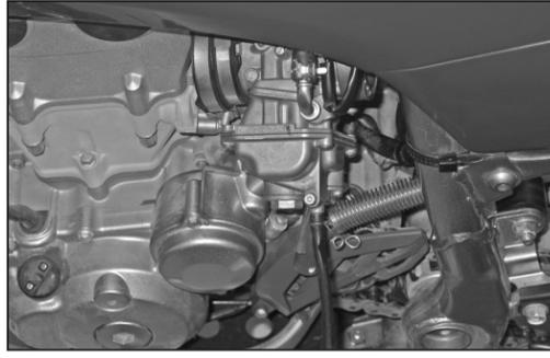
13. Disconnect the crank case vent hose from the vent fitting. Loosen the hose clamp which secures the carburetor to manifold hose; disconnect the carburetor from the manifold and pull it out to the side of the chassis as shown.
