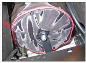
23. Secure the filter mounting bracket to the filter with the hardware provided. Then secure the tube to the silicone hose with the hose clamp provided.
