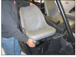
2. Release the locking lever and remove the two passenger seats from the vehicle.
