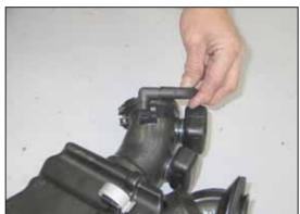
15. Remove the carburetor slide vent hose and 90° fitting from the stock intake tube as shown.
