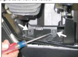
4. Remove the front two air box retaining clips shown.
