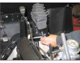
8. Release the shifter drain hose clamp and remove the drain hose from the shifter assembly as shown.
