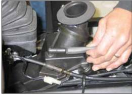
6. Unhook the crank case vent hose from the factory air box as shown.
