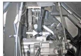
10. Install the filter mounting bracket onto the engine boss as shown with the provided hardware. **NOTE: Do not completely tighten at this time.**
