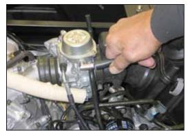
5. Unhook the carburetor slide vent hose from the carburetor as shown.
