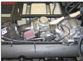
25. Install the crank case vent hose onto the crank case vent filter as shown.
