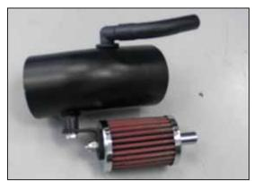
18. Install the crank case breather assembly onto the K&N® intake tube as shown with the provided hardware.
