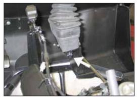
9. Install the supplied nylon plug onto the shifter drain tube and secure with factory clamp.
