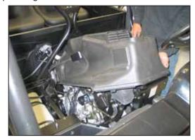
3. Unhook the engine cover, lift and remove the engine cover from the vehicle.
