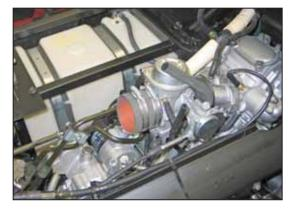
11. Install the silicone hose (08284) onto the carburetor and secure with the provided hose clamp.
