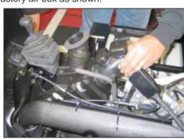
7. Loosen the hose clamp that secures the intake tube to the carburetor and then remove the complete intake system as shown.
