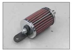
17. Install the "L" bracket (070066) onto the K&N  $^{\!\otimes}$  crank case breather filter as shown.
