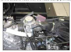
24. Install the carburetor slide vent hose onto the carburetor port as shown.
