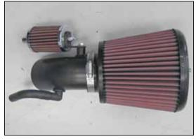
19. Install the K&N® air filter onto the intake tube assembly and secure with the provided hose clamp.
