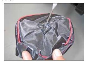
20. Using a sharp instrument, poke a hole in the center of the reinforcement patch of the K&N® Drycharger®.
