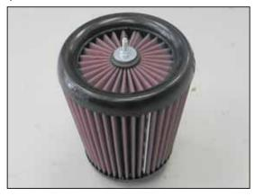
13. Install the supplied ¼-20 bolt through the filter top and secure with the supplied rubber washer, fender washer, and standard nut as shown.
