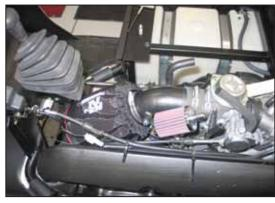
22. Install the K&N® intake assembly into the silicone hose at carburetor and align with the filter mounting bracket installed during step #9.
