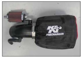
21. Install the K&N® Drycharger® onto the K&N® air filter.
