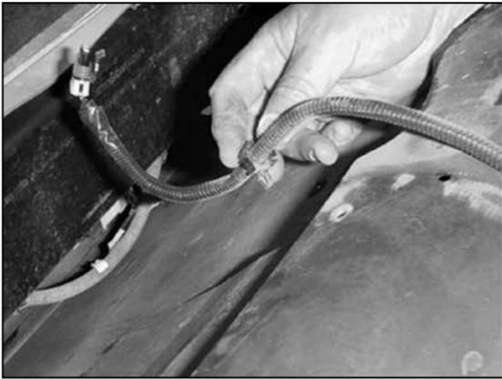
8. Detach the wiring harness retaining clip from the lower radiator cover.
