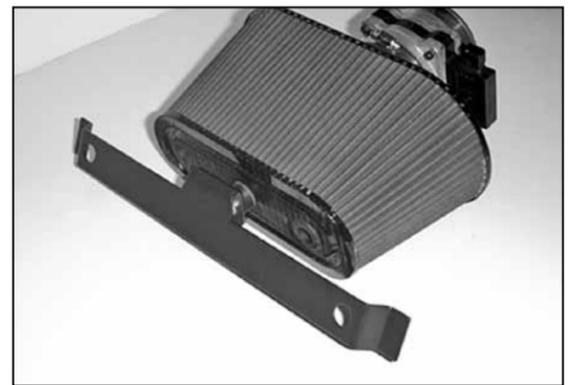
20. Attach the angled bracket to the rubber mounted stud using the provided hardware.
