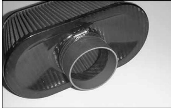
13. Attach the 3.75" ID silicone hose (08621) onto the flange of the Air filter element.
