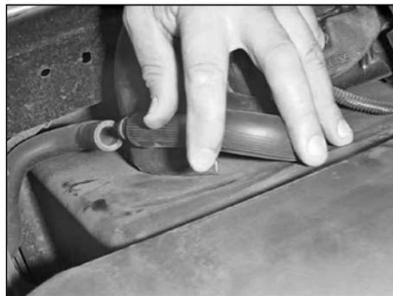
3. Disconnect the air injection vent hose.
