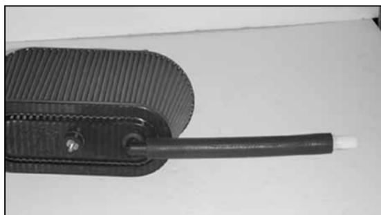
17. Insert the 90 degree vent into the grommet in the top plate of the filter.
