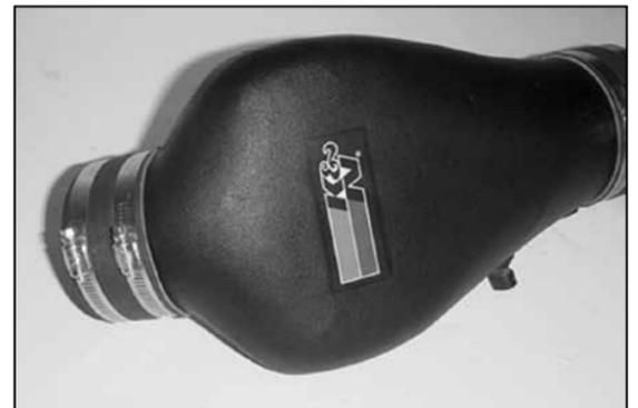
19. Install a 3.5" ID silicone hose (08630) onto the K&N® intake tube.
