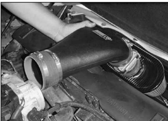
47. Reinstall the K&N® intake assembly then adjust the radiator cover for best fit under the intake tube, then tighten the 4 retaining bolts.
