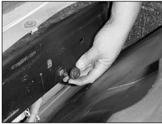
12. Remove the two grommets from the airbox mounting points.
