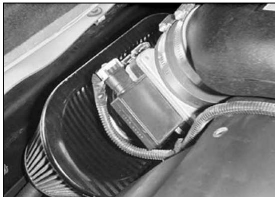
51. Reconnect the mass air sensor electrical connection.
