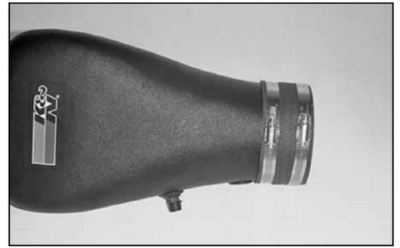
18. Install the 4" ID silicone hose (08755) onto the K&N® intake tube.
