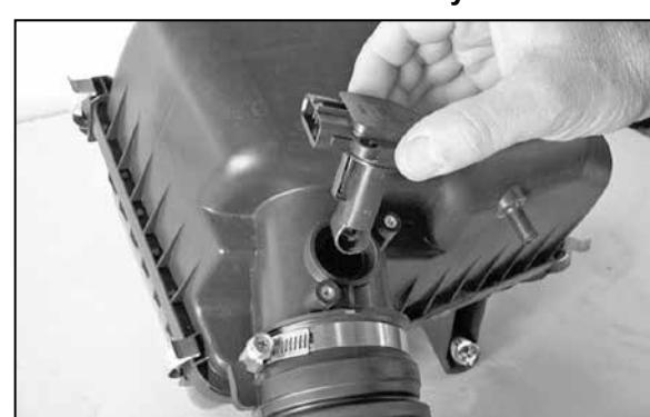
8. Loosen and remove the screws that secure the mass air sensor, then remove the mass air sensor.
