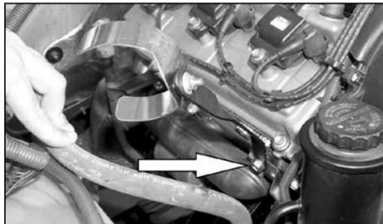
19. Install the saddle bracket assembly onto the motor using the bolt from step 18. Do not tighten completely.
