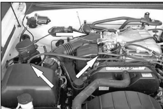
3. Disconnect the three hoses from the air box resonator and intake hose.
