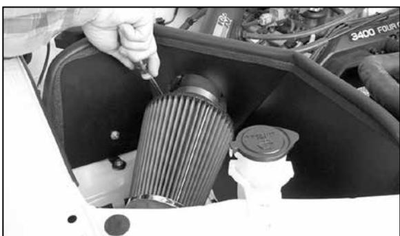
29. Install the K&N® Filter onto the K&N® intake tube and secure it with the provided hose clamp.
