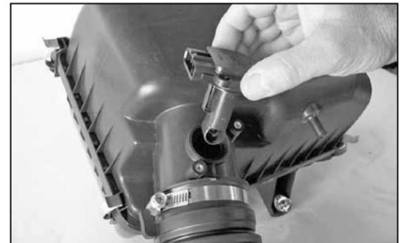
8. Loosen and remove the screws that secure the mass air sensor, then remove the mass air sensor.
