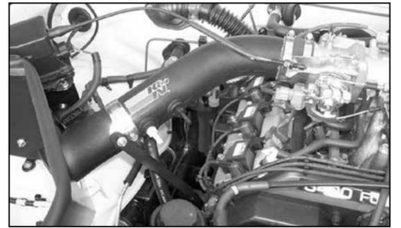
22. Install the K&N® intake tube onto the throttle body then tighten the hose clamps at the throttle body and saddle bracket.
