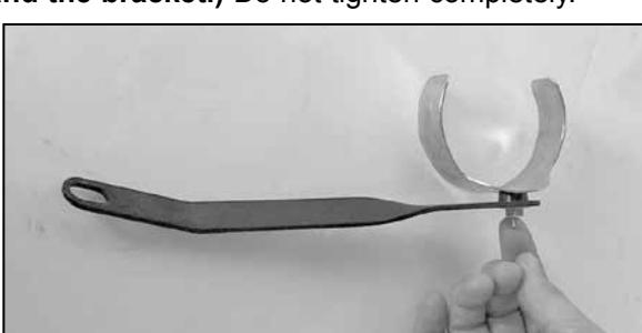
15. Assemble the saddle bracket as shown.
