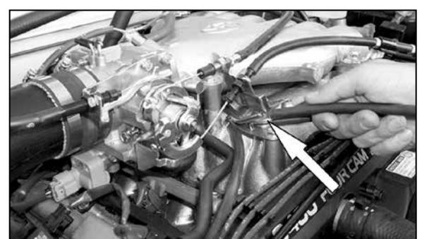
25. Remove the rubber hose from the intake manifold as shown.
