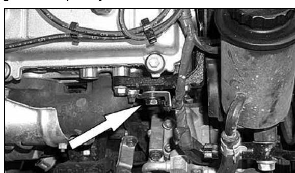
18. Loosen and remove the bolt that secures the wire harness bracket located directly behind the power steering reservoir.
