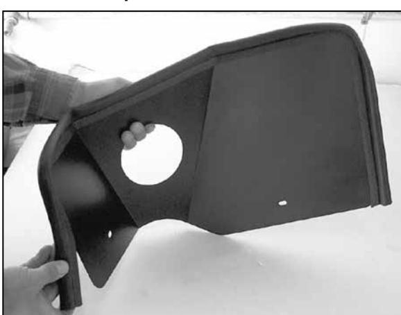
12. Install the edge trim onto the heat shield as shown above. Trim if needed.
