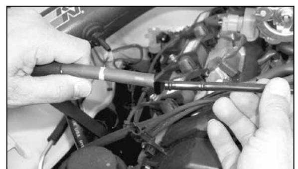
23. Remove the rubber hose from the hard plastic vent line as shown.
