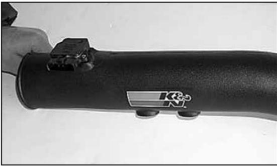
10. Using the provided screws and spacers install the mass air sensor into the K&N® intake tube as shown above.
