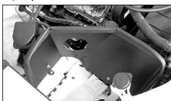
20. Install the heat shield and secure it to the new K&N® brackets with the hardware provided. Do not tighten completely.
