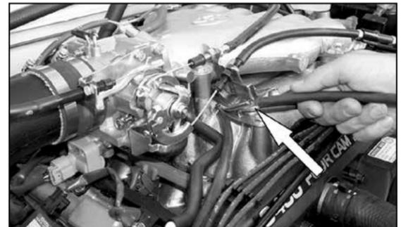
25. Remove the rubber hose from the intake manifold as shown.
