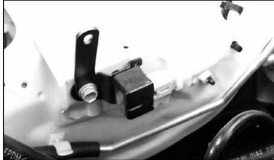
17. Install the bracket onto the relay bracket using the bolt that was removed in step 16. Do not tighten completely.
