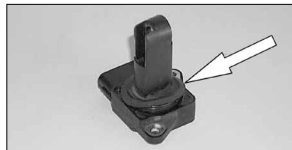
9. Apply the provided gasket to the mass air sensor with the sticky side down.
