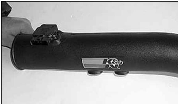
10. Using the provided screws and spacers install the mass air sensor into the K&N® intake tube as shown above.
