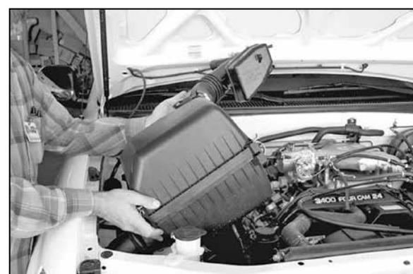
7. Remove the complete air intake system.
