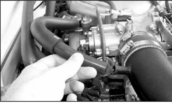
28. Connect the silicone hose to the crankcase vent line then connect the silicone hose to the K&N® intake tube as shown.
