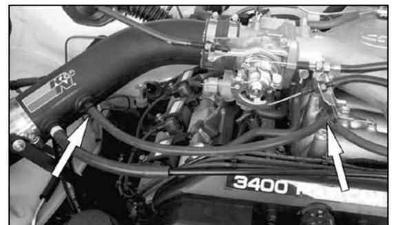
26. Install the new silicone hose onto the K&N® intake tube and then install the other end onto the intake manifold as shown.
