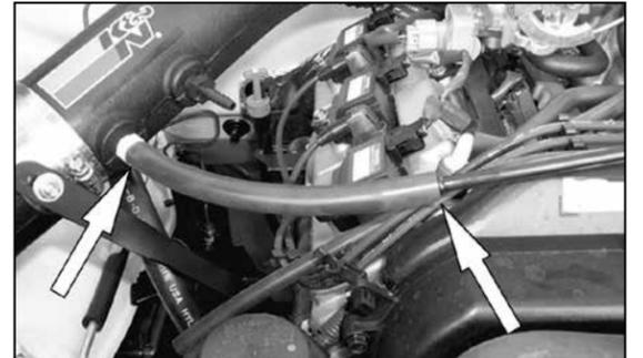
24. Install the provided silicone hose onto the K&N® intake tube and connect the other end to the hard vent line as shown.
