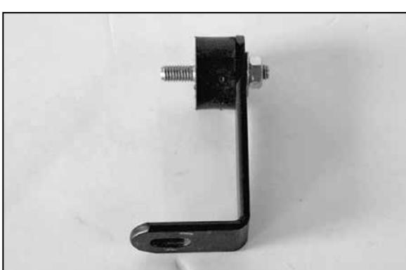
13. Assemble the "L" bracket and rubber mounted stud as shown.
