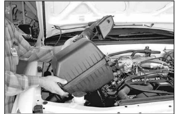
7. Remove the complete air intake system.
