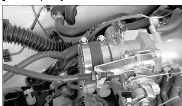
21. Install the silicone hose and hose clamps onto the throttle body as shown.
