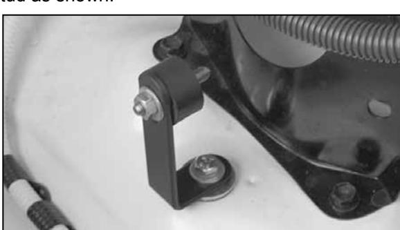
14. Install the "L" bracket onto the existing air box mounting hole. (**NOTE: Rubber washer & fender washer should be mounted between the fender and the bracket.**) Do not tighten completely.
