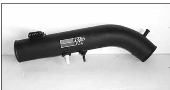
11. Install the provided vents into the K&N® intake tube.
