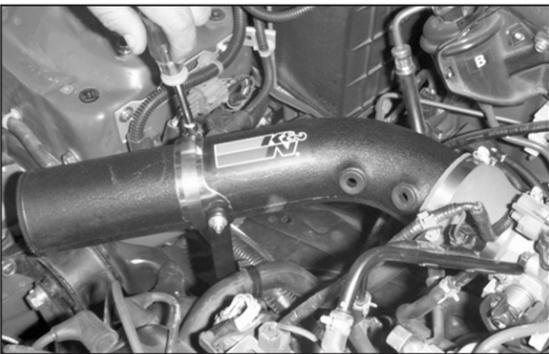
13. Secure the K&N® intake tube to the saddle bracket with the hose clamp provided.
