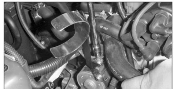
9. Install the saddle bracket assembly between the wiring harness bracket and support bracket, then secure with the hardware provided.
