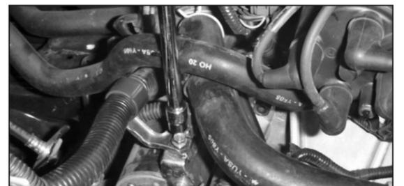
7. Loosen and remove the bolt that secures the wiring harness bracket to its support bracket.
