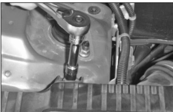
3. Loosen and remove the two bolts that secure the airbox.
