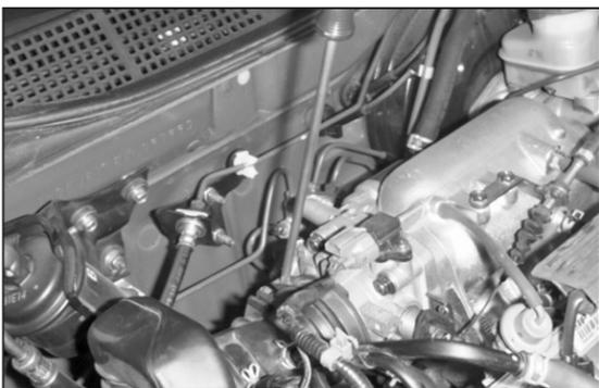
2. Loosen the hose clamp on the intake tube at the throttle body.
