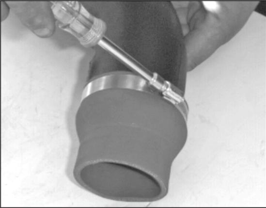
11. Install the silicone adapter onto the K&N® intake tube.
