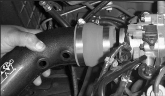
12. Install the intake tube onto the throttle body and secure it with the provided hose clamp.
