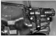
18. Carefully unscrew & remove the IRV from the side of the air box.
