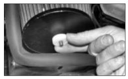
16. Fit the studded lid of the filtercharger to the slotted hole in the front of the heat shield using the plastic spacer supplied.
