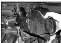
4. Remove the 2 torx head bolts from the air box, carefully remove the air box from the vehicle.
