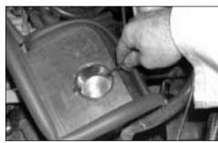
10. Pierce/drill two holes in the top of the flexi cold air hose to match the holes in the bottom of the heat shield. Attach the flexi hose to the hole in the bottom of the heat shield using 2 plastic ties supplied.
