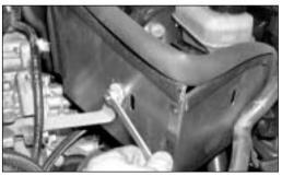
9. Secure the heat shield to the mounting bracket using a allen head bolt, nylock nut & washers supplied.
