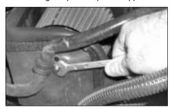
17. Secure the coolant reservoir hose to the front of the heat shield using a 'P' clip supplied. Set the height of the filtercharger on the slotted hole, then secure using a nylock nut & washer supplied.
