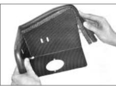
8. Clip the edge trim seal to the outside edge of the heat shield as shown (trim any excess seal).
