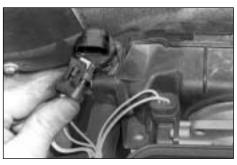
3. Remove the rubber hose & electrical harness plug from the IRV (idle regulator valve).
