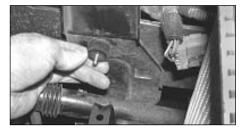
5. Remove the bolt securing the air box support frame to the chassis leg, replace the bolt with the studded rubber mounting supplied.
