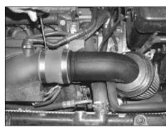
11. Ovalise the end of the stepped silicon hose on the new intake assembly & fit it to the original plastic intake housing using a #44 hose clip supplied.
