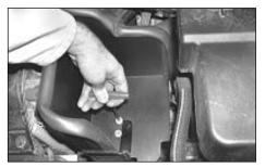
8. Attach the heat shield to the 'S' shaped bracket using the short allen head bolts, nylock nuts & washers supplied.
