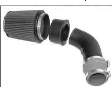
10. Fit the stepped silicon hose & rubber filter adapter onto new intake pipe. Fit the new Filtercharger to the intake pipe / filter adapter, fully tighten the hose clips supplied.
