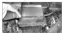
3. Carefully lift the complete air box assembly out of its mounting rubbers & remove the assembly from the car.
