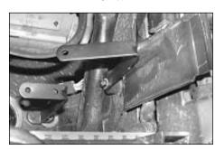
6. Attach the new angled bracket to the studded rubber mounting using a nylock nut & small washer.
