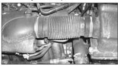
2. Unclip & remove the flexi intake hose from the plastic housing.
