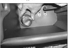
9. Carefully expand the flexi cold air hose, remove one of the plastic hose ends & insert the hose through the hole in the heat shield. Feed the hose down to the lower spoiler.
