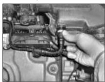
5. Squeeze together the yellow tabs located on the end of the engine breather pipe, unclip & remove the breather pipe from the air box.
