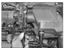
4. Unclip & remove the intake pipe from the throttle housing
