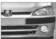
10. Feed the flexi cold air hose down to the lower grille, secure the hose to the grille using a plastic tie supplied.
