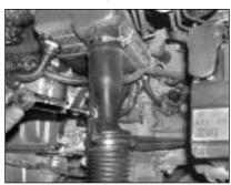
3. Remove the bolt securing the intake pipe to the support bracket.
