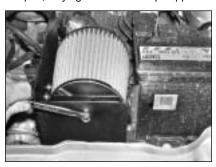
15. Fit the studded lid of the filtercharger to the slotted hole in the front of the heat shield using the plastic spacer, nylock nut & washer supplied.
