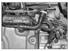
7. Remove the engine breather pipe from the breather 'T' piece, it may be necessary to cut the pipe away from the 'T' piece, taking the necessary safety precautions.
