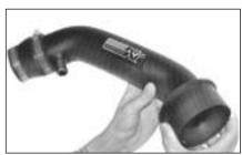
11. Fit the stepped adapter hose to the end of the new plastic intake pipe using a #48 clip supplied, attach the rubber filter adapter to the other end of the intake pipe.
