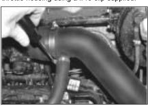
13. Fit the new breather hose between the breather 'T' piece & intake pipe using the #12 clips supplied.
