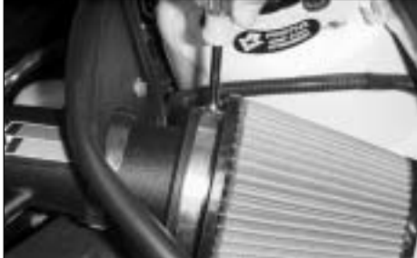
21. Install the Filtercharger® onto the intake tube.
