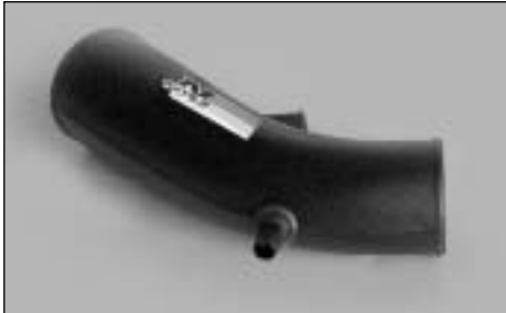
16. Install the air temperature sensor into the new intake tube.
