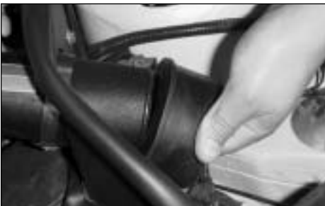
20. Install the filter adapter onto the intake tube.
