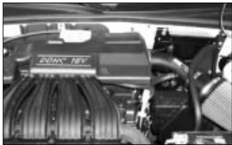
24. Install the engine cover back onto motor.
