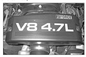
35. Install the stock throttle body cover and fasten using the stock nuts.
