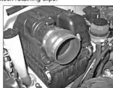
27. Install the provided silicone hump hose onto the air box and fasten with the provided hose clamp.
