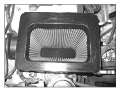
25. Install the K&N® air filter into the lower air box.
