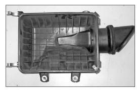
23. Re-install the fresh air duct into the lower air box and fasten with the provided hardware.
