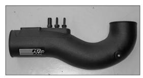
10. Install the three provided 1/4" npt fittings into the  $K\&N^{\odot}$  intake tube as shown.
