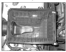
24. Re-install the lower air box into it's stock location and fasten with the stock hardware.
