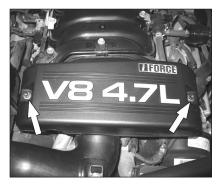
3. Remove the two nuts that fasten the throttle body cover, then remove the throttle body cover.
