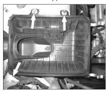
18. Remove the stock air filter, then remove the three bolts that secure the lower air box to the inner fender.
