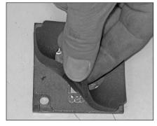
11. Install the provided gasket onto the K&N $^{\!0}$  mass air sensor adapter.
