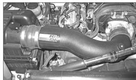
28. Install the K&N® intake tube into the silicone hoses previously installed onto the throttle body and air box.
