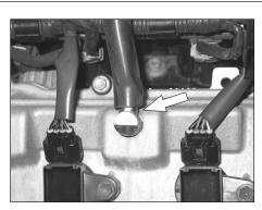
7. Disconnect the crank case vent hose from the valve cover.
