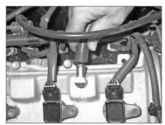
33. Install the remaining open end of the crank case vent hose onto the stock fitting on the valve cover.
