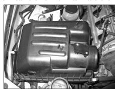
26. Install the upper air box and fasten with the stock retaining clips.
