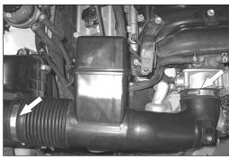
8. Loosen the hose clamps that fasten the stock intake tube to the throttle body and air box.
