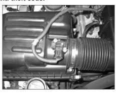
2. Disconnect the mass air sensor electrical connection, then release the mass air sensor wiring harness from the air box.
