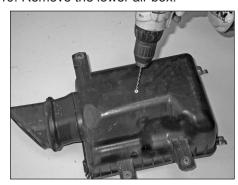
20. Drill out the center of the rivet that fastens the fresh air duct to the lower air box, then remove the rivet.
