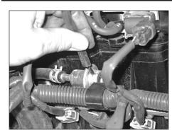
30. Connect the remaining open end of the 4mm silicone hose to the fuel pressure regulator vent port.
