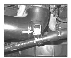
4. Remove the bolt that fastens the A/C mounting clamp.
