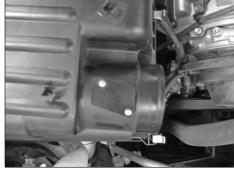
13. Install the provided mass air sensor block off plate onto the stock air box.
