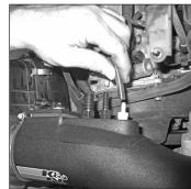
29. Install the provided 4mm silicone hose onto the npt vent fitting previously installed onto the K&N® intake tube.
