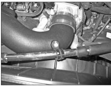
34. Fasten the A/C hose mounting clamp to the K&N<sup>®</sup> intake tube using the stock mounting bolt removed in step #4.
