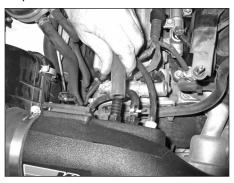
32. Install the provided crank case vent hose onto the npt fitting previously installed into the K&N® intake tube.
