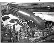
9. Remove the stock intake tube.
