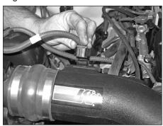
36. Re-connect the mass air sensor electrical connection.
