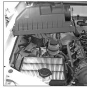
17. Release the four upper air box retaining clips, then remove the upper air box.
