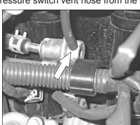
6. Disconnect the fuel pressure regulator vent line from the fuel pressure regulator.
