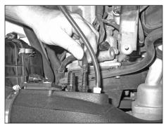
31. Connect the P/S pressure switch vent hose to the npt fitting previously installed into the K&N® intake tube, then fasten using the stock spring clamp.
