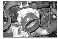
16. Install the provided silicone hose onto the throttle body and fasten using the provided hose clamp.
