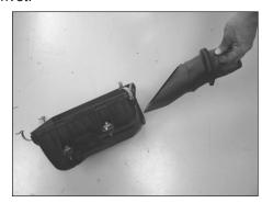
21. Remove the fresh air duct from the lower air box.
