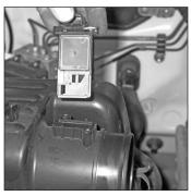
12. Remove the two screws that fasten the mass air sensor to the stock air box, then remove the mass air sensor.
