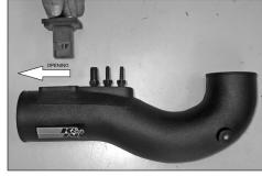
15. Install the mass air sensor assembly into the K&N® intake tube and fasten with the provided hardware.
