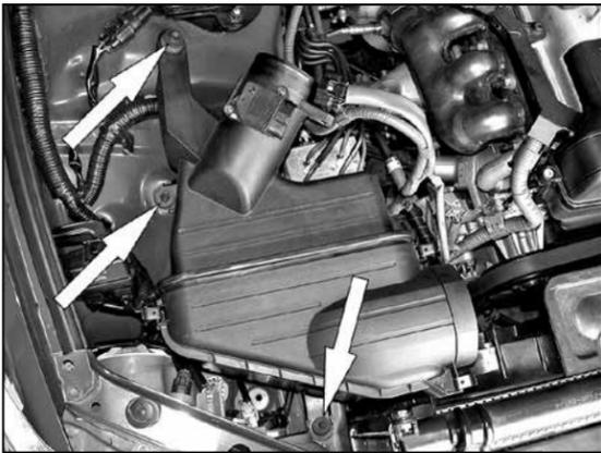
9. Remove the 3 bolts that retain the air box onto the vehicle.
