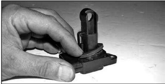
23. Install the provided gasket onto the mass air sensor with the sticky side towards the mass air.
