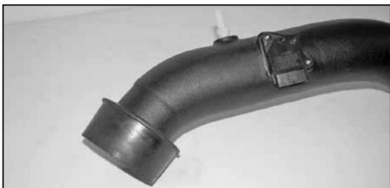
26. Install the filter adapter onto the K&N® intake tube as shown.
