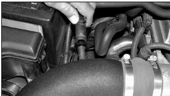
32. Reconnect the crank case vent as shown.
