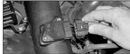
35. Reconnect the mass air electrical sensor as shown.
