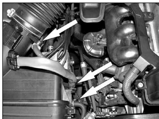
4. Remove the 3 clips that retain the electrical harness onto the factory air box.
