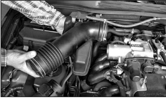
7. Remove the intake tube as shown.
