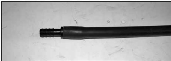
28. Install hose mender into the provided silicone hose as shown.
