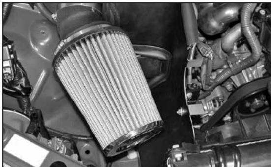
33. Install the K&N® Air Filter onto the intake tube as shown.
