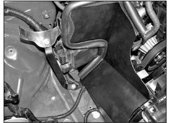
20. On 01 models, mount the heat shield and saddle bracket assembly onto the vehicle with the provided 8mm button head bolt as shown.
