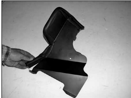
16. Install edge trim onto the heat shield as shown. Trim if needed.
