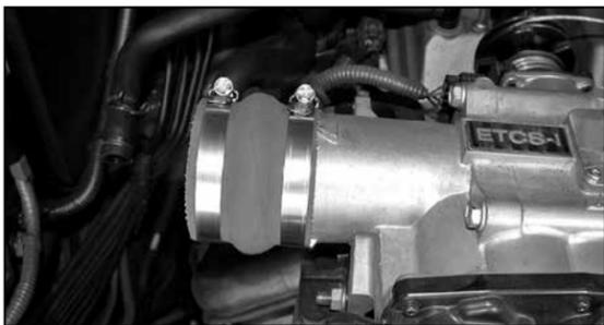
25. Install the hump hose onto the throttle with the provided hose clamps.
