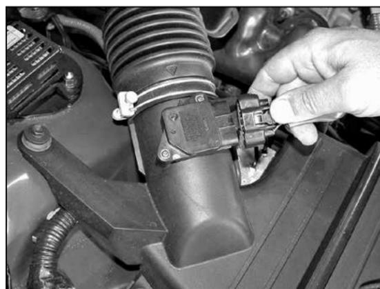
3. Disconnect the mass air electrical connection.
