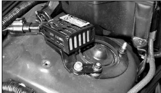
15. Install the new K&N® bracket onto relay and then onto strut mount as shown. Tighten all hardware completely.
