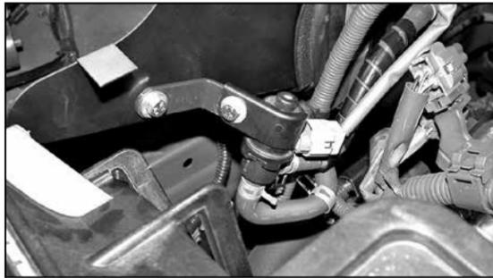
29. Mount the "L" bracket onto the heat shield and then mount the evap solenoid onto the bracket with the provided hardware.
