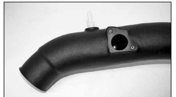
21. Install the vent fitting onto the new K&N® intake tube as shown.
