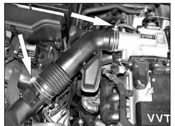
6. Loosen the 2 hose clamps that secure the intake tube to the air box and the throttle body.
