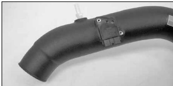
24. Install the mass air onto the new K&N® intake tube with the provided hardware as shown.
