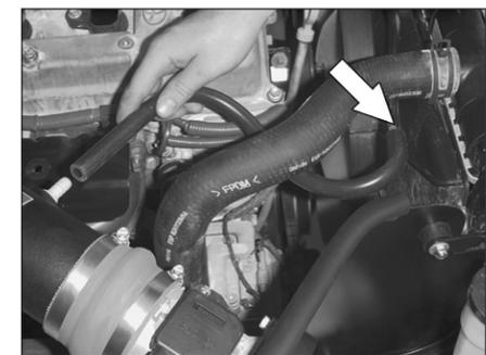
25. Install the provided silicone hose onto the EVAP canister vent and secure the other end onto the K&N® intake tube as shown.
