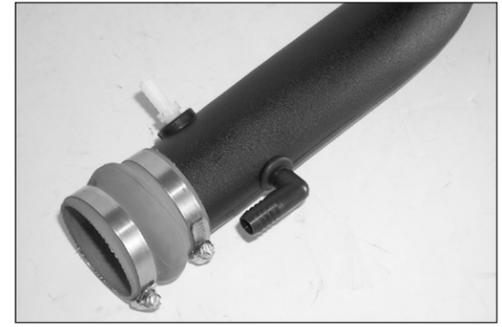
21. Install the 90 degree fitting into the intake tube as shown.
