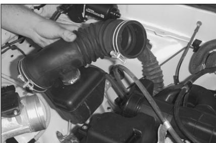
3. Loosen the two hose clamps on the intake hose and remove the intake hose as shown.
