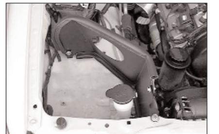
17. Install the heat shield and secure it to the new K&N® brackets with the hardware provided as shown. Do not tighten completely.
