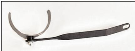
14b. On 2000-02 vehicles, assemble the saddle bracket as shown above.
