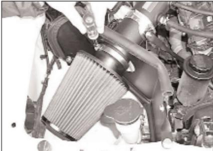
22. Install the K&N® air filter onto the K&N® intake tube and secure it with the provided hose clamp. **NOTE: Drycharger® air filter wrap; part # RC-4700DK is available to purchase separately. To learn more about Drycharger® filter wraps or look up color availability please visit <http://www.knfilters.com>.**
