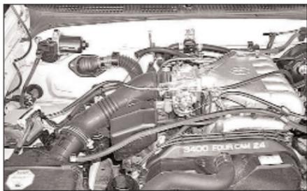
3. Disconnect the three hoses from the air box resonator and intake hose.
