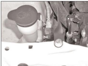
13. Install the twist bracket onto the existing air box-mounting hole with the provided hardware as shown. Do not tighten completely.
