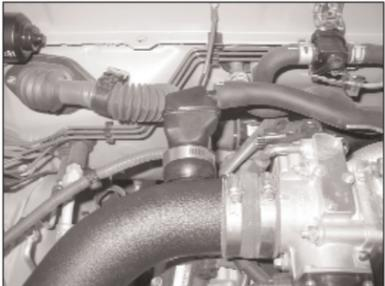
21a. On vehicles equipped with crank case vent resonator, connect the factory crank case vent hose onto the resonator as shown. **NOTE: The crank case vent hose may need to be repositioned to enable it to reach the resonator.**
