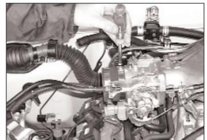
18. Install the silicone hose and hose clamps onto the throttle body as shown.
