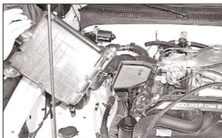
6. Remove the complete air intake system.
