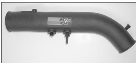
10a. On models that come equipped with one vent line install provided plug into the K&N® intake tube as shown.
