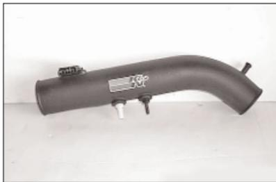
10. Install the provided vents into the K&N® intake tube.
