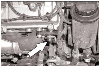
15. On 1999-2002 vehicles loosen and remove the bolt that secures the wire harness bracket located directly behind the power steering reservoir.
