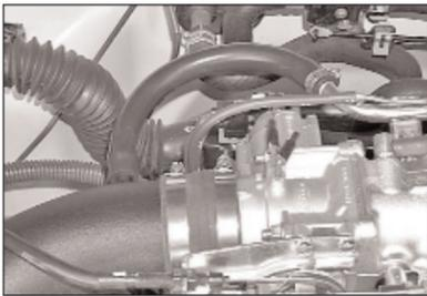
21. On 1999-00 models, attach the provided silicone hose onto the crankcase vent and connect it to the K&N® intake as shown.
