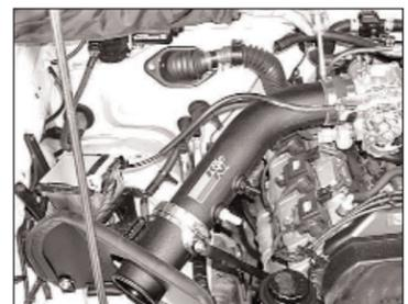
19. Install the K&N® intake tube onto the throttle body, and then tighten the hose clamps at the throttle body and saddle bracket.
