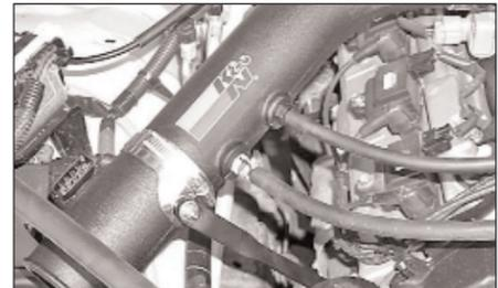
20. Install the provided silicone hose onto the engine and connect it to the K&N® intake tube as shown then attach the vent line to the evap canister to the K&N® intake tube as shown.
