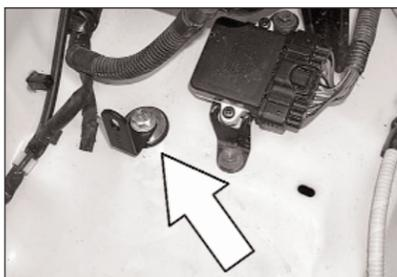
12. Install the "L" bracket onto the existing air box-mounting hole.
