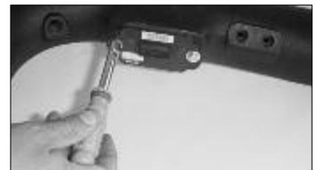
13. Install the provided bushings into the mass air sensor as shown.
