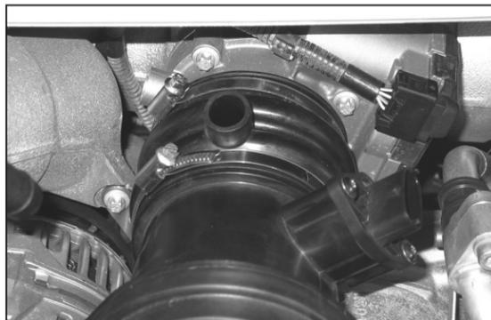
6. Loosen the hose clamp securing the factory intake tube to the throttle body as shown. Pull the factory intake tube from the throttle body.
