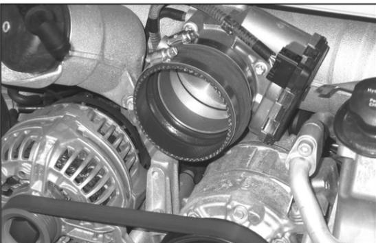
15. Install silicone hose (#08699) onto the throttle body and secure with the provided hose clamp as shown.
