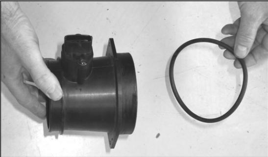
12. Remove the "O" ring seal from the mass air sensor housing as shown.
