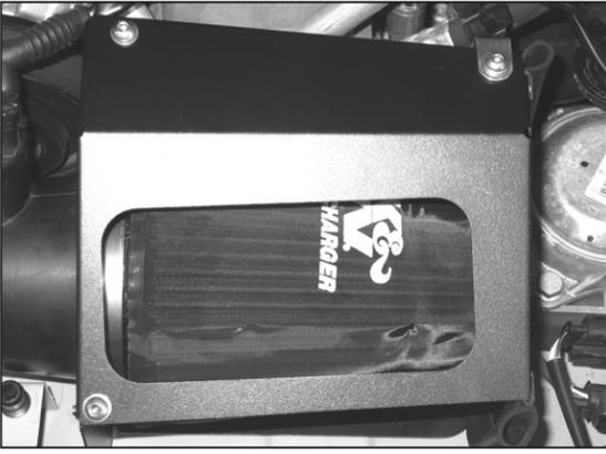
27. Install the heat shield top cover and mass air sensor harness clip (removed in step # 4) onto the heat shield with the provided hardware as shown.
