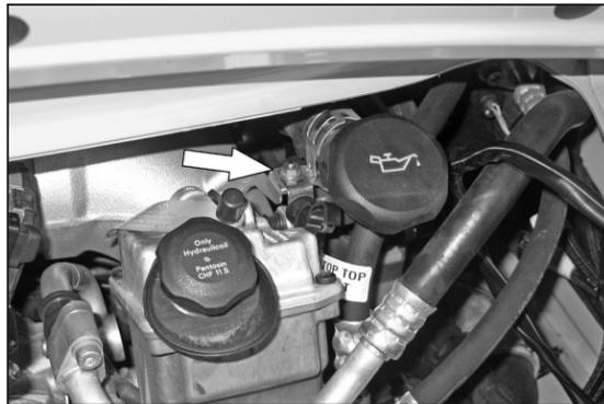
4. Remove the 10mm nut securing the harness clip, then remove the harness clip as shown. Re-install the 10mm nut and tighten. Set the harness clip aside for use in a later step.
