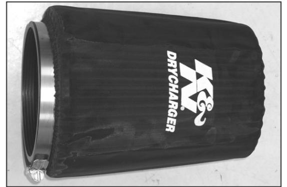
24. Install the provided K&N® Drycharger® onto the K&N® air filter as shown.
