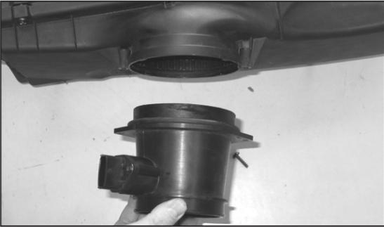
11. Remove the two torx screws that secure the mass air sensor to the factory air box. Remove the mass air sensor housing as shown.
