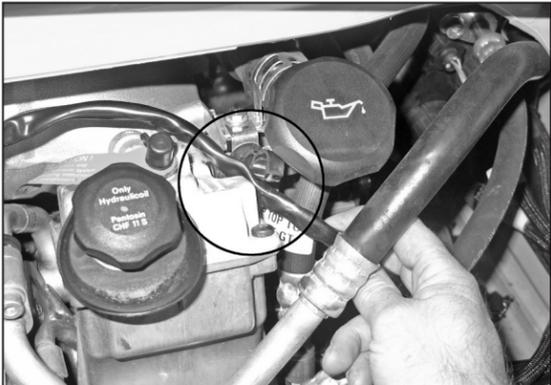
3. Release the mass air sensor clip (near the oil filler cap) as shown.
