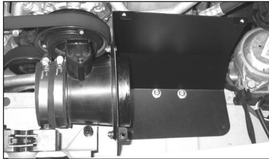
18. Install the heat shield assembly onto the heat shield bracket with the provided hardware as shown.
