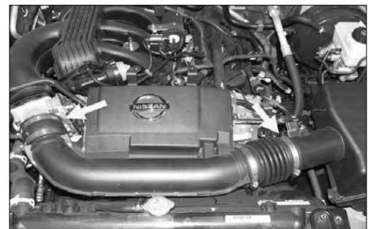
7. Loosen the two hose clamps shown which secure the stock intake tube to the air box and to the throttle body.
