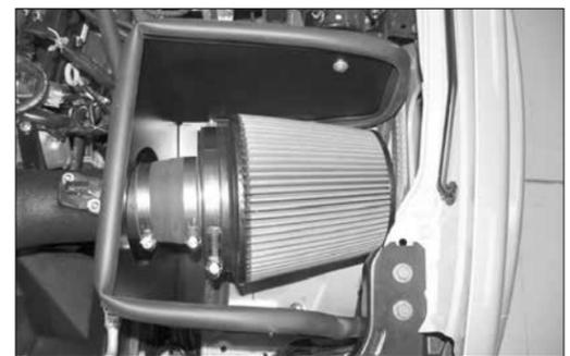
27. Install the air filter assembly onto the K&N® intake and secure with the provided hose clamp.
