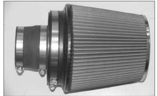
26. Install the silicone hose (08051) onto the air filter assembly as shown and secure with the hose clamp.
