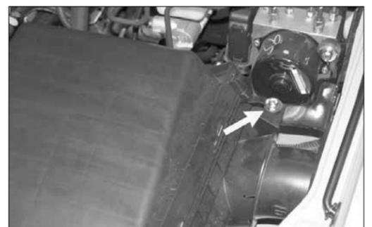
9. Remove the air box retaining bolt shown.
