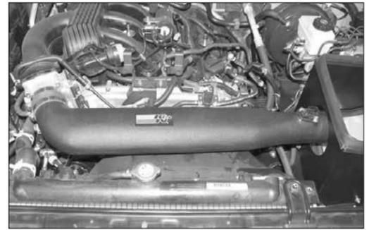
23. Install the K&N® intake tube into the silicone hose at the throttle body and align with the mounting bracket installed onto the heat shield. Secure the intake tube with the provided hardware.
