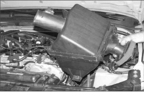
10. Pull firmly on the air box to dislodge it from the mounting grommets and remove it from the vehicle.
