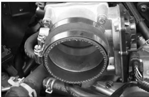
20. Install the silicone hose (08434) onto the throttle body and secure with the provided hose clamp.
