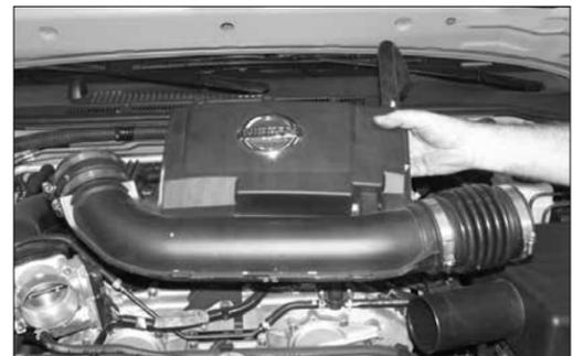
8. Remove the intake tube from the vehicle as shown.
