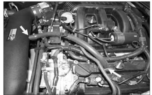
24. Attach the provided crank case vent hose to the valve cover and K&N® intake tube as shown and secure with the provided hose clamps.
