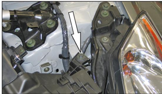
5. Remove the air box mounting bolt, which secures the air box to the inner fender.
