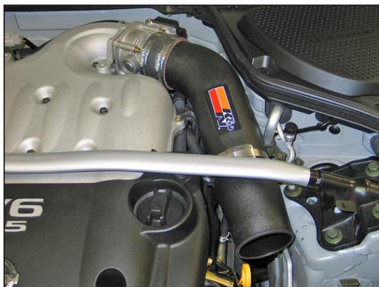
18. Install the K&N® intake tube onto the throttle body and saddle clamp and then secure with the provided hose clamps as shown.
