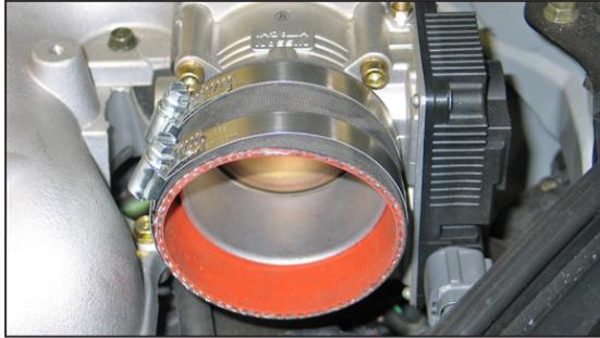
17. Install the provided silicone hose (08690) onto the throttle body with the provided hose clamps as shown.
