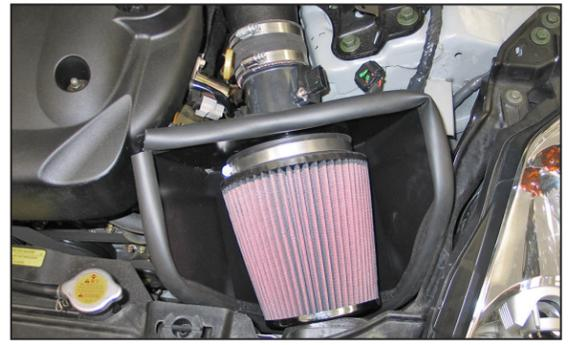
21. Install the Air Filter / mass air sensor assembly onto the K&N® intake tube, slide the silicone hose onto the mass air sensor housing and secure with the provided hose clamp as shown.
