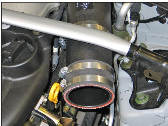
19. Install the silicone hose (08690) onto the end of the K&N® intake tube with the provided hose clamps.
