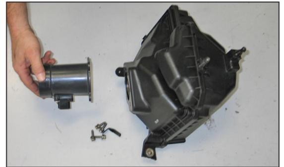
8. Remove the four bolts, which secure the mass air sensor to the factory air box and then separate the mass air sensor from the air box.
