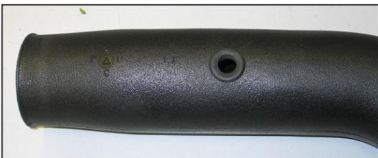
15. Install the provided grommet into the K&N® intake as shown.
