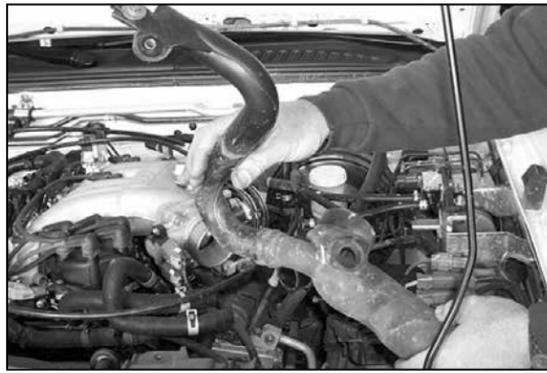
16. Remove the front resonator assembly as shown.
