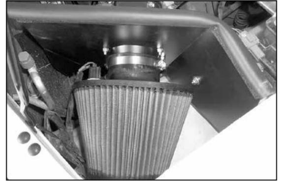
39. Install RX-4750 air filter element and secure with hose clamp using an 8mm socket or nut driver. **NOTE: Drycharger® air filter wrap; part # RF-1042DK is available to purchase separately. To learn more about Drycharger® filter wraps or look up color availability please visit <http://www.knfilters.com>.**
