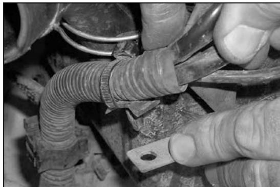
18. Using pliers, remove the wire loom clip.
