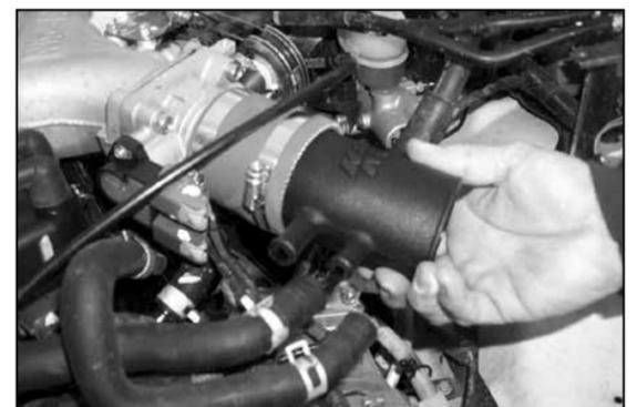
26. Install hose clamp #48 and the intake tube onto the silicone hose on the throttle body. Do not tighten completely.
