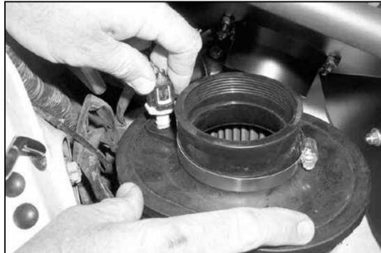
38. Insert air temp sensor into base of air filter.
