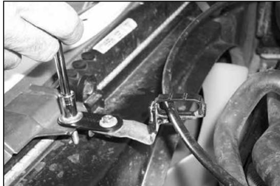
37. Reconnect the throttle cable bracket using the flat bracket, two washers, 10mm bolt, nylock nut and the stock bolt. Tighten completely.
