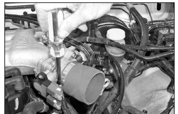
25. Install silicone hose, (08096), and hose clamp #44 onto the throttle body and tighten.
