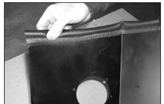
27. Install edge trim seal onto heat shield as shown.
