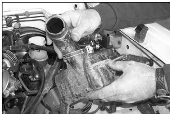
19. Remove the resonator box as shown.
