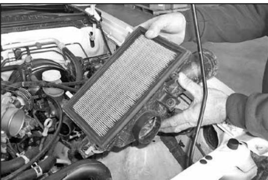
13. Remove the lower air filter housing as shown
