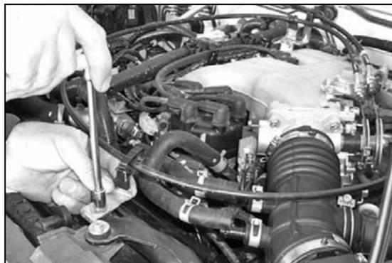
6. Disconnect the cruise control cable bracket using a 10mm socket.
