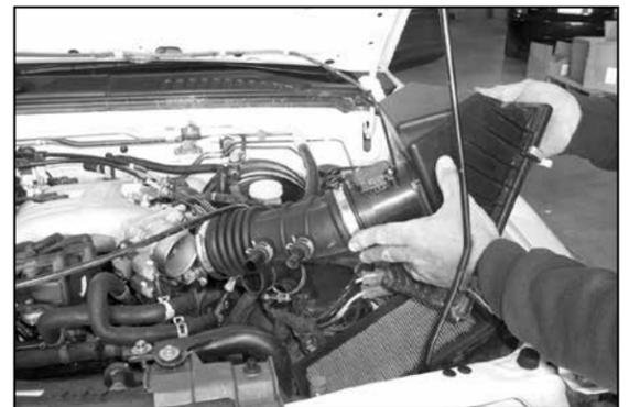
9. Unlatch the four clips on the air filter housing and remove the top assembly.
