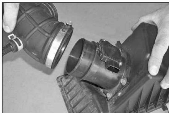
20. Loosen hose clamp using a 10mm socket and remove air duct tube from mass air sensor.
