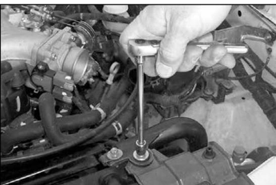
15. Remove bolt from front of resonator using a 10mm socket.
