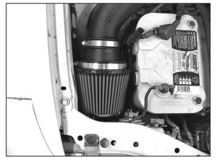
8. Install the K&N® filter onto the filter adapter; secure with the provided hose clamp. If needed, slightly adjust/move the "L" bracket at both the filter adapter and inner airbox mounting nut in order to obtain the best fit.
