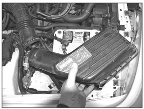
3. Lift the air box lid up; then, disconnect the stock intake tube from the air box lid.
