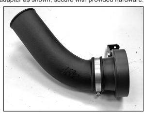
6. Install the filter adapter into the K&N® intake tube; position as shown and secure with the provided hose clamp.
