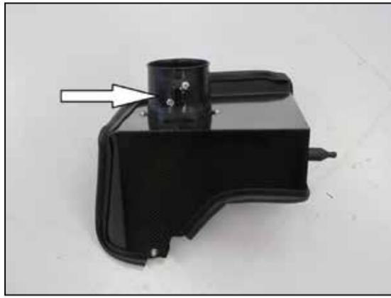
12. Install the mass air sensor into the K&N® mass air sensor housing and secure with the provided hardware.
