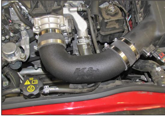
11. Install the K&N® intake tube into the coupling hose on the air box and then into the hose on the throttle body. Secure the tube with the provided hose clamps.
