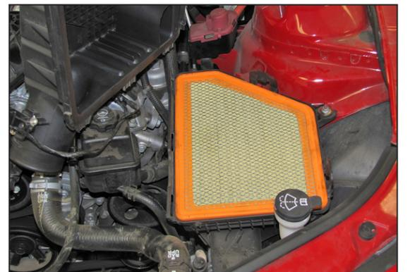
5. Releases the upper air box cover latches' and lift off the upper air box, then remove the factory air filter.
