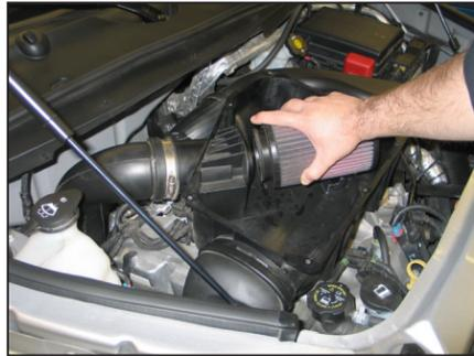
3. Remove the stock air filter from the air box as shown.
