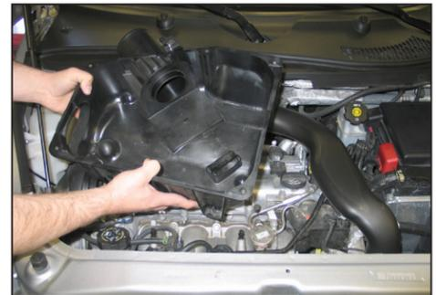
7. Remove the two clips securing the front of the air box to the engine and then remove the complete air box assembly from the vehicle.
