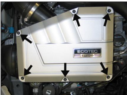
2. Remove the six TORX screws which secure the air box lid and then remove the air box lid from the vehicle.
