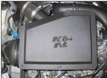
18. Install the K&N® air box lid and secure with the six factory screws.
