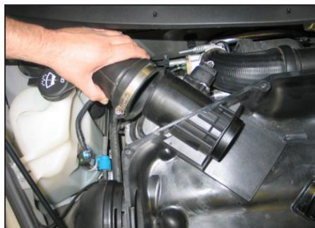
5. Loosen the hose clamp and then disconnect the stock intake tube from the air box.
