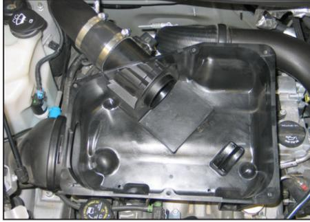
15. Install the air box onto the engine, connect the intake tube and secure with the provided hose clamp. Reinstall the retaining clips to secure the front of the air box. Reconnect the fresh air inlet tube to the air box.
