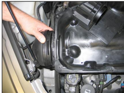
4. Disconnect the fresh air inlet duct from the air box as shown.
