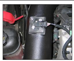
25. Reconnect the mass air sensor electrical connection.
