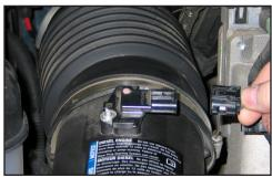
2. Depress the locking tab and then disconnect the Mass air sensor electrical connection.
