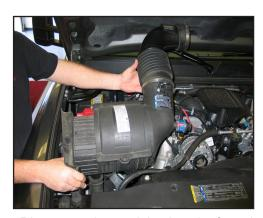
4. Disconnect the stock intake tube from the turbo inlet tube and then lift the complete stock intake assembly from the vehicle as shown.
