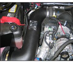
21. Install the K&N® Intake Tube into the silicone hose at the turbo inlet and into the heat shield, then secure the K&N® Intake Tube with the provided hose clamp and hardware as shown.
