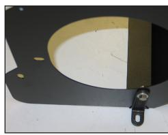
15. Install the "L" bracket (07805) onto the heat shield as shown with the provided hardware.
