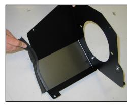
17. Install one of the 11" edge trims onto the heat shield as shown.
