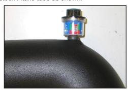
14. Install the filter minder and grommet into the  $K\&N^{\otimes}$  Intake Tube as shown.
