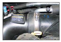
3. Loosen the hose clamp which secures the stock intake tube to the turbo inlet tube.
