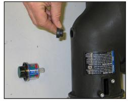
13. Remove the filter minder and grommet from the stock intake tube as shown.
