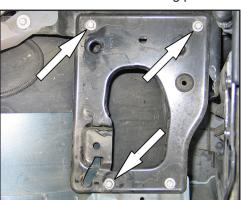
7. Remove the three air box mounting plate bolts shown.
