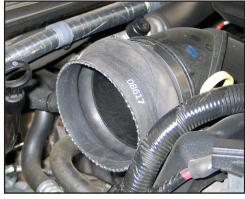
5. Install the provided silicone hose (08617) onto the turbo inlet tube and secure with the provided hose clamp.
