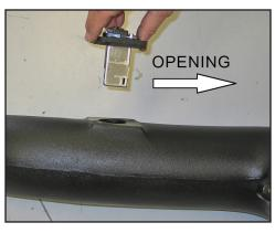
11. Install the mass air sensor assembly into the  $K\&N^{\otimes}$  Intake Tube.
