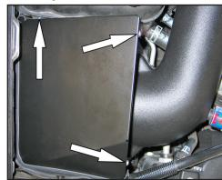
24. Install the filter cover onto the heat shield and secure with the provided hardware.
