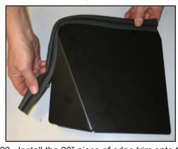
23. Install the 20" piece of edge trim onto the filter cover as shown.
