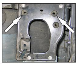
6. Remove the two air box mounting grommets shown from the air box mounting plate.
