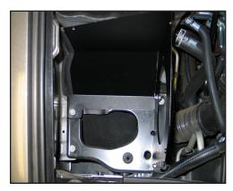
19. Install the Heat shield assembly onto the factory air box mounting plate and secure with the factory bolts removed in step #7.
