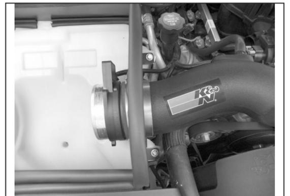
27. Install the mass air sensor assembly onto the intake tube and secure with the hose clamp provided.
