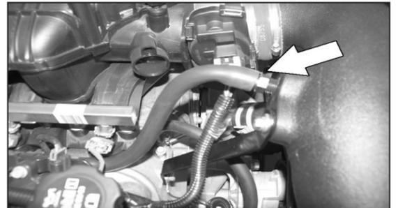
25. Connect the supplied crankcase vent hose onto the valve cover and then connect to the intake tube as shown.
