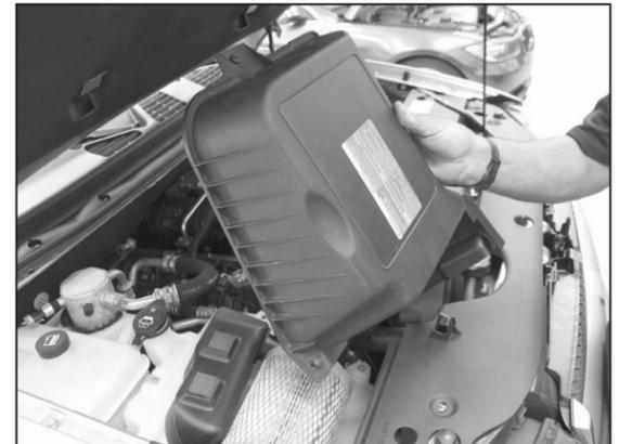
8. Lift up on the core support cover for clearance and then remove the airbox lid as shown.
