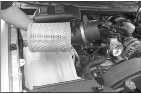
10. Remove the filter and mass air sensor assembly from the vehicle as shown.
