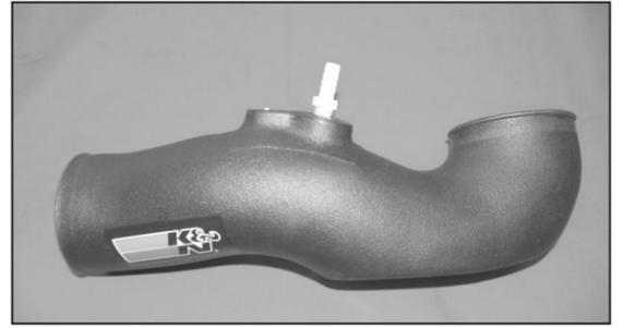
23. Install the provided vent fitting into the intake tube as shown.
