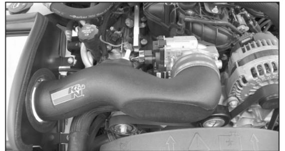
24. Install the intake tube into the silicone hose at the throttle body and align with the mounting bracket installed in step #20. Secure the tube with the provided hose clamp and hardware. Do not completely tighten at this time.
