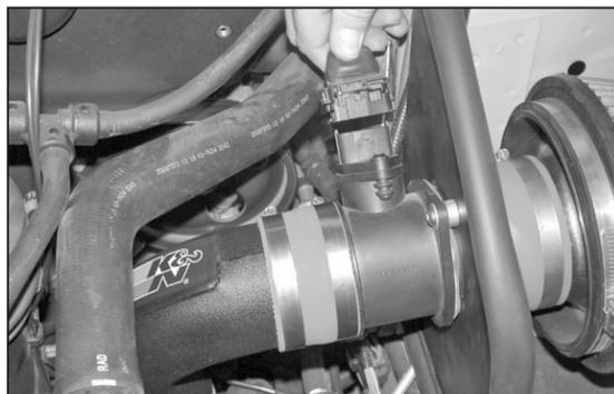
18. Reconnect the mass electrical connection as shown.
