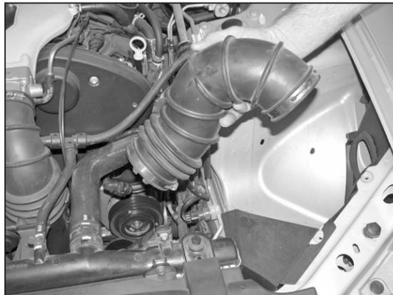
5. Loosen the lower hose clamp on the intake tube, then remove intake tube as shown.
