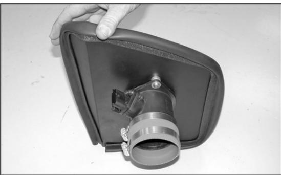
13. Install silicone hose (08434) onto the mass air assembly with the provided hose clamps as shown.
