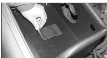
25. Apply the gasket provided onto the heat shield to cover the exposed bolts.
