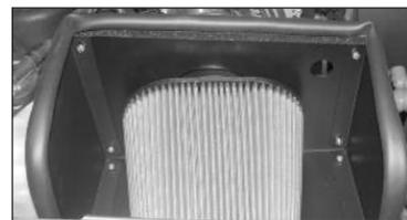
35. Install the K&N® air filter element and secure with the provided hose clamp.
