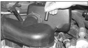
2. Loosen and remove the tall wing nut on the throttle body.
