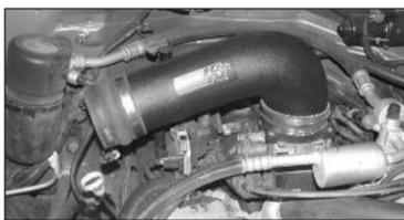
28. Install the intake tube onto the silicone hose at the throttle body.
