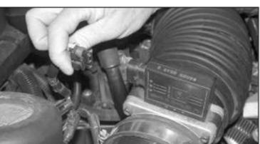
6. Disconnect the mass air sensor electrical connection
