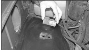
9. Using a 13mm socket, remove the lower air box bracket from the inner fender.
