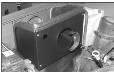
24. Install the heat shield assembly and secure to the inner fender using the hardware provided.
