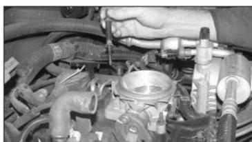
10. Remove the stock intake tube mounting bolt from the throttle body.
