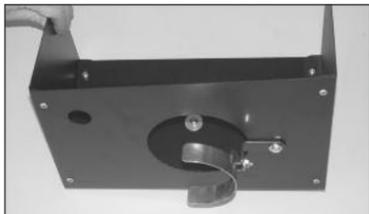
22. Install the saddle bracket assembly to the heat shield using the hardware provided.
