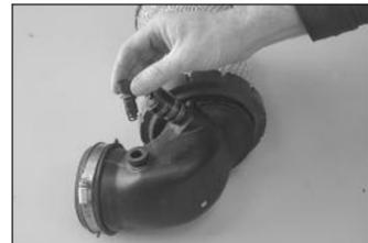
14. Remove the air temperature sensor from the factory intake tube.
