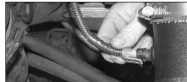
36. Reconnect the mass air sensor and air temp sensor electrical connections.
