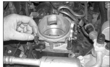
15. Hand tighten the three provided coupling nuts on the original throttle body studs.
