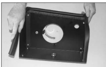
23. Install the trim seal onto the heat shield. **NOTE: Some cutting and trimming will be necessary for best fit.**
