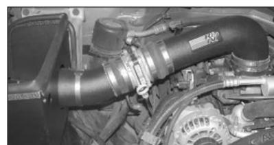
34. Install the primary tube/mass air assembly onto the secondary intake tube and heat shield saddle clamp and secure with the provided hose clamps.
