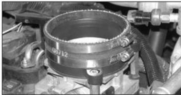
27. Install silicone hose (08712) onto the throttle body adapter and secure with the provided hose clamp as shown.
