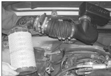
7. Lift and remove the complete air intake system.
