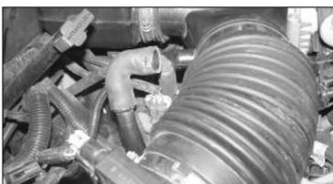
4. Disconnect the crank case vent hose from the factory air intake tube.
