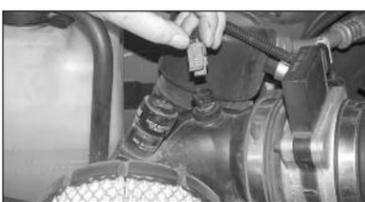
5. Disconnect the air temperature sensor electrical connection.
