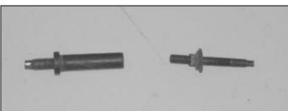
11. Using a 5/16" wrench, remove the factory bolt from the stand off and reinstall the factory bolt in its original location.
