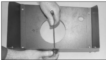
20. Install the rubber mounted studs onto the bottom of the heat shield using the hardware provided.
