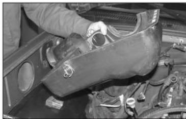
8. Remove the lower air box assembly.
