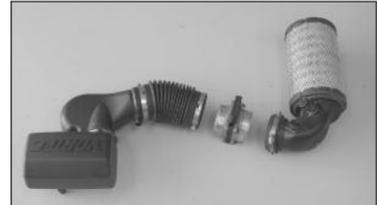
13. Using a flat blade screwdriver, loosen the hose clamps and remove the mass air sensor from the stock intake tube.
