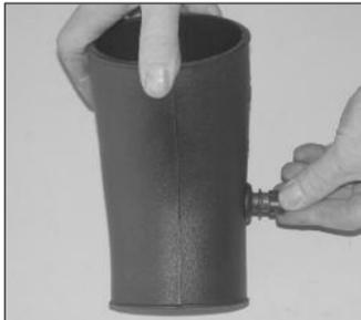
32. Install the air temp sensor into the primary intake tube as shown.
