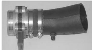
33. Install the primary intake tube assembly onto the mass air sensor assembly and attach with the provided hose clamp as shown.
