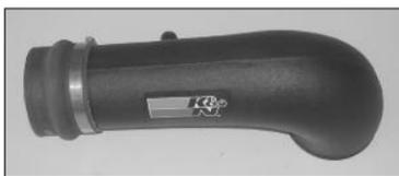
26. Install the silicone hump hose (08699) onto the secondary intake tube and secure with the hose clamp as shown.
