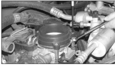
17. Install the throttle body adapter and hand start the three 6mm allen bolts.
