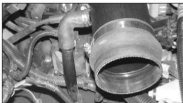
29. Install the crank case vent onto the secondary intake tube and secure with the provided hardware.
