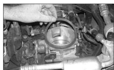
16. Install the neoprene gasket provided onto the throttle body flange.
