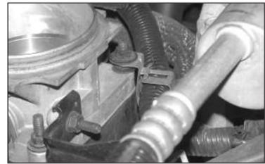
12. Using a 10mm socket remove the wire harness retaining clip nut at the front of the throttle body.
