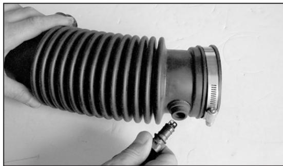
17. Remove the air temp sensor from stock intake tube as shown.
