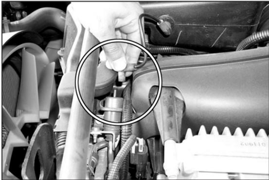
2. On vehicles equipped with a fuel pressure regulator vent, disconnect the vent hose from the fuel pressure regulator as shown.
