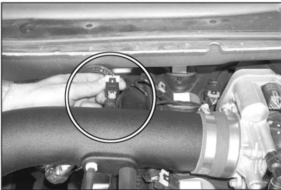
23. Reconnect the air temp. electrical connection as shown.
