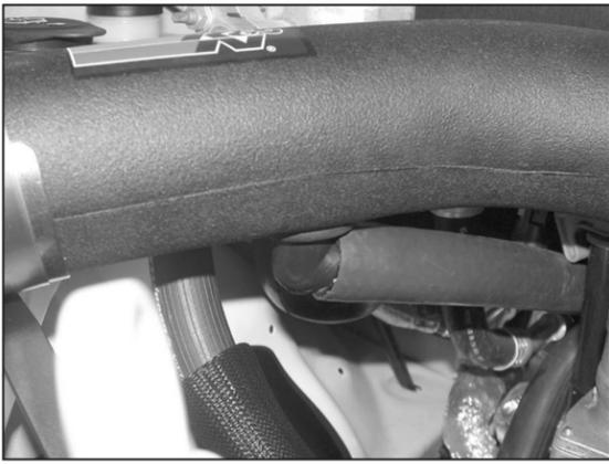
20d. Re-install the intake tube onto the vehicle, then install the 90 degree fitting into the grommet on the intake tube as shown.
