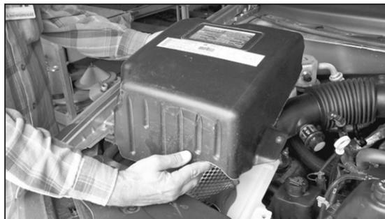
4. Remove the upper airbox cover from vehicle as shown.
