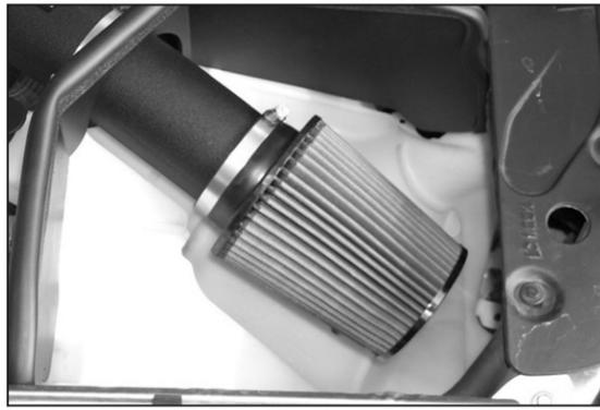
24. Install the K&N® Air Filter onto the K&N® intake tube as shown.
