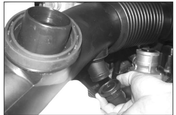
5a. On vehicles with air injection squeeze release ring then remove air injection line from intake tube.
