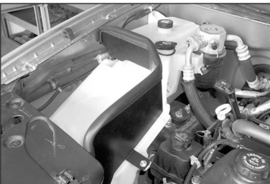
11. Install heat shield into vehicle using the hardware provided.
