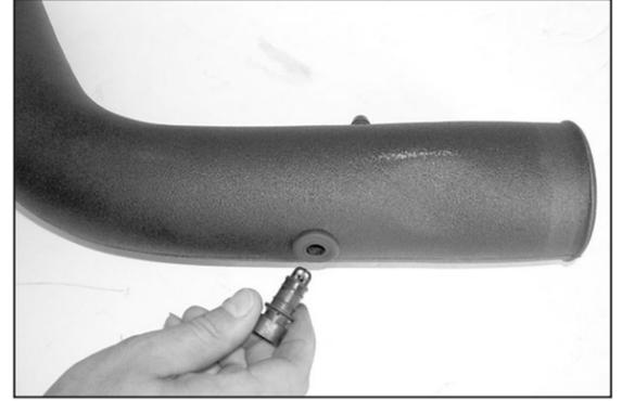
19. Install the air temp sensor into the new K&N® intake tube as shown.
