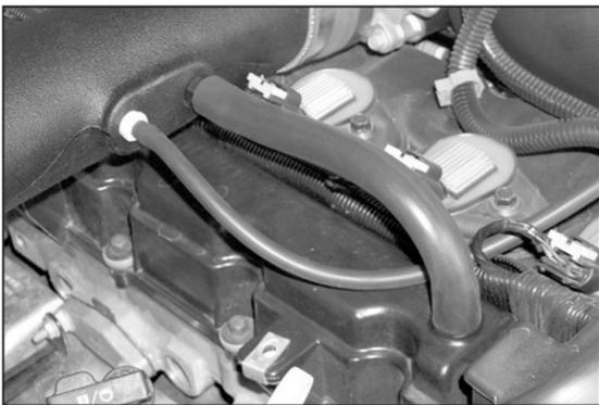
22. Install the 1/2" silicone hose onto the K&N® intake tube and the other end onto the crankcase vent as shown.
