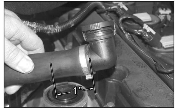
20a. On vehicles with air injection cut the vent hose 1" from end of hose.
