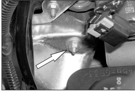
13. Remove the nut that secures the exhaust heat shield to cylinder head as shown.
