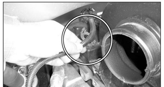
7. Disconnect the clip that holds the air temp. electrical connection wiring loom then remove the wire loom.
