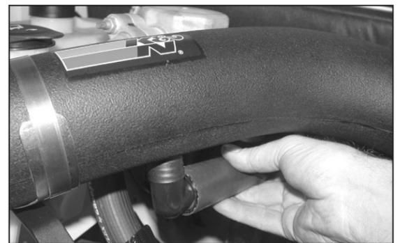
20b. On vehicles with air injection install the 90 degree fitting into the vent line then mark the intake tube where the fitting lines up with tube, then remove intake tube from vehicle.
