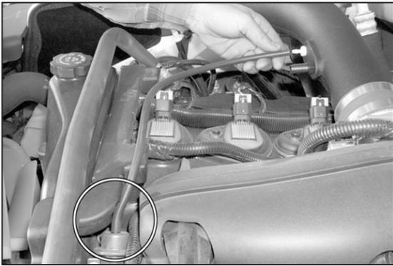
21. On Vehicles equipped with a fuel pressure regulator vent hose, install the provided 4mm silicone hose onto the K&N® intake tube and the other end onto the fuel pressure regulator vent as shown.
