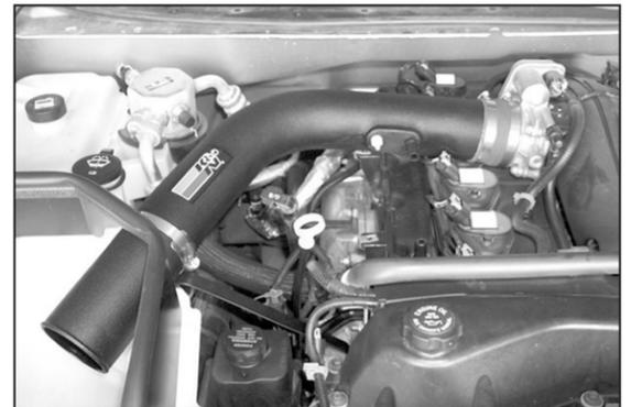
20. Install the new K&N® intake tube into the vehicle and tightening hose clamp at the throttle body and at the saddle bracket as shown.
