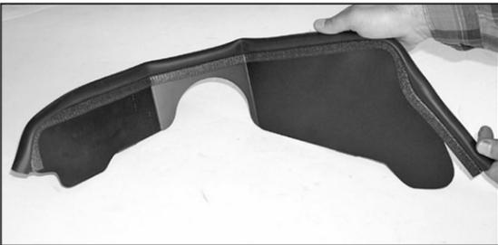
10. Install edge trim onto the heat shield as shown. Trim if needed.
