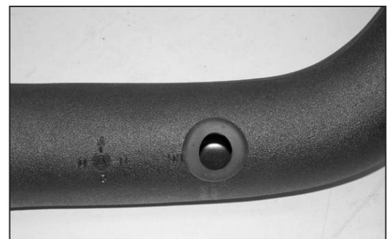
20c. Use a 1-1/4 hole saw and drill a hole where the intake tube was marked in the previous step. Then install the provided grommet as shown.
