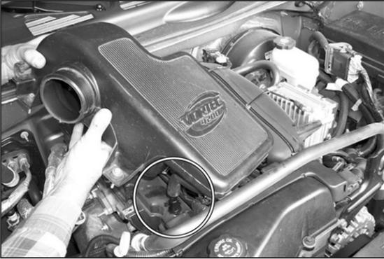
9. Remove the intake resonator from vehicle as shown.
