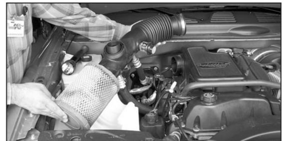
6. Loosen hose clamp at intake resonator then remove complete air intake tube.
