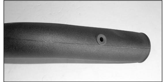
18. Install the provided grommet onto the new K&N® intake tube as shown.
