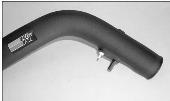
16. Install the provided vent fittings onto the K&N® intake tube as shown.
