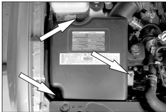
3. Loosen and remove the three screws that retain the upper airbox cover.
