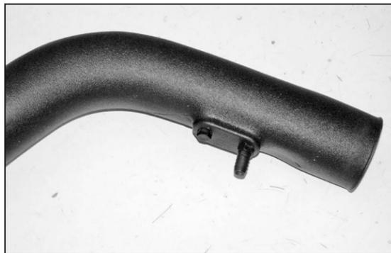
16a. On vehicles not equipped with a fuel pressure regulator vent use the npt pipe plug provided in place of the 3/16" barbed fitting.
