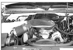
3. Loosen the hose clamps at the throttle body and at the mass air sensor, then remove the factory intake tube as shown.
