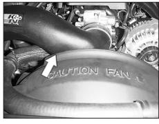
13. Due to production tolerances it may be necessary to mark the fan shroud as indicated, remove the intake tube and trim the fan shroud.
