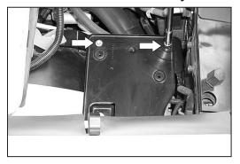
5. Loosen and remove the two air cleaner mounting tray bolts as shown.
