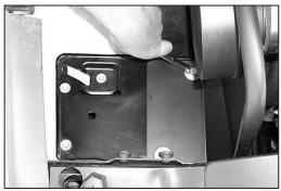
14. Adjust the heat shield and intake tube for best fit, then tighten the two hex bolts as shown.
