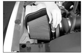
15. Install the K&N® air filter onto the heat shield assembly as shown.
