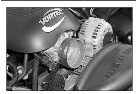
10. Install the silicone hose and hose clamps onto the throttle body as shown.
