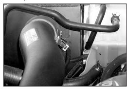
16. Reconnect the mass air sensor electrical connection as shown.
