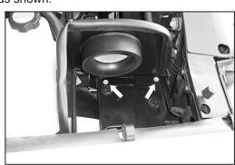
9. Install and mount the heat shield assembly to the air cleaner mounting tray using the bolts removed in step 5.
