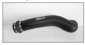
11. Install the silicone hump hose and hose clamps onto the K&N<sup>®</sup> intake tube as shown.
