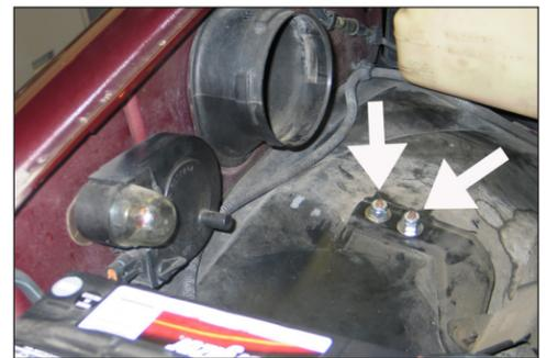
5a. On vehicles equipped with rear A/C-heat, secure the heater hose manifold bracket to the inner fender with the factory bolts removed in step #5 and the nuts provided.
