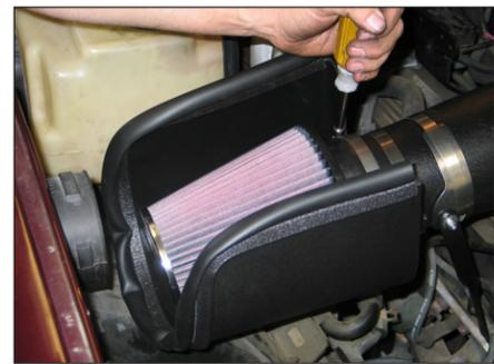
21. Install the K&N® air filter onto the intake tube as shown.
