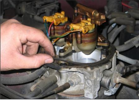
7. Remove the factory air cleaner gasket.
