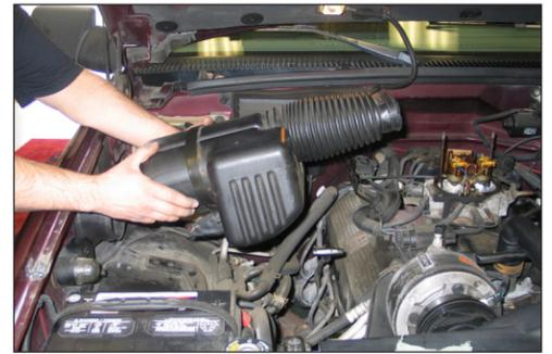
5. Loosen and remove the two bolts that secure the air inlet/resonator, then, remove the complete assembly.
