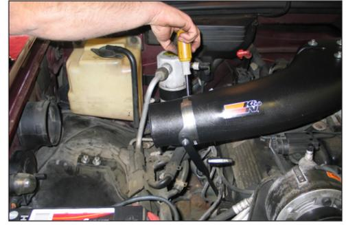
18. Secure the tube to the saddle bracket assembly using the provided hose clamp.
