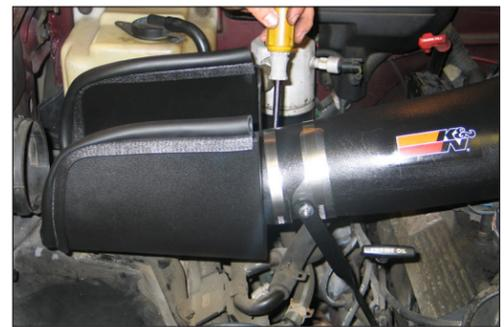
20. Install the heat shield onto the tube as shown, but do not tighten completely.
