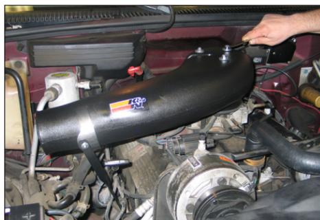
17. Re-install the K&N® intake tube and secure it with the provided washers and nylock nuts.
