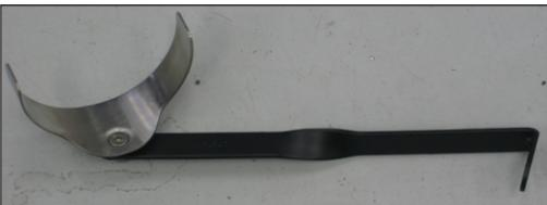
10. Assemble the saddle bracket assembly as shown.
