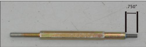
8a. Apply two drops of the provided thread locker to the provided 5mm studs, then install the studs into the tube mounting studs as shown so that .750" is exposed.
