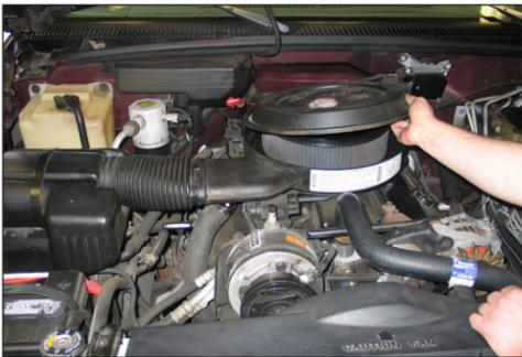
2. Loosen and remove the air cleaner wing nuts, then remove the air cleaner lid.
