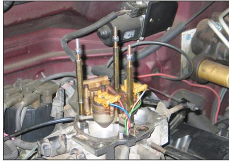
13. Apply the three nylock nuts onto the throttle body studs as shown approximately 3/4" down.
