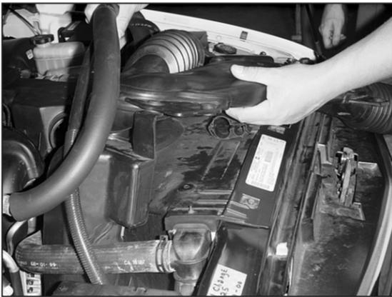
9. Remove the entire intake tube assembly.
