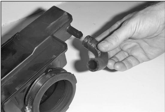
27. Detach the O.E. crankcase vent hose from the resonator.
