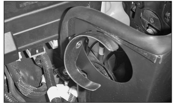
22. Install the saddle bracket assembly onto the airbox mounting stud and secure using the hardware provided.
