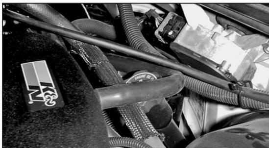
33. Attach the vent hose to the vent fitting on the intake tube.
