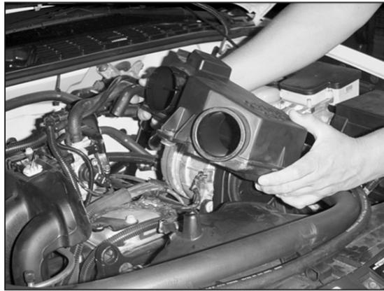
15. Detach the resonator from the throttle body and remove it.
