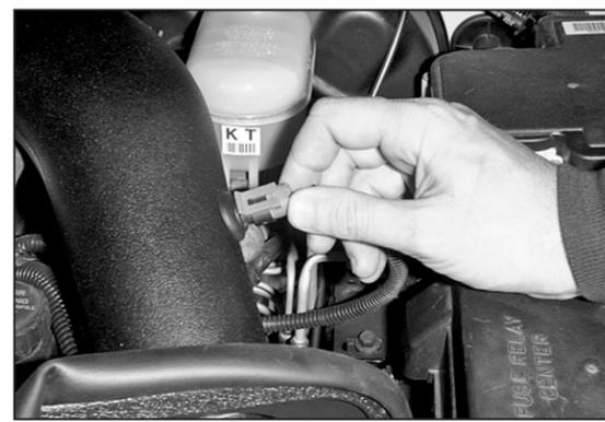
37. Reconnect the air temperature sensor electrical connection.
