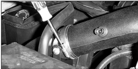
32. Secure the saddle bracket to the intake tube using the hose clamp provided.
