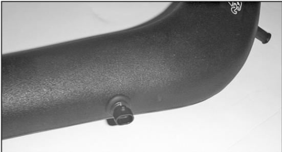
25. Install the air temperature sensor into the grommet in the K&N® intake tube.
