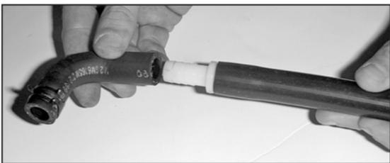
28. Connect the O.E. crankcase vent hose and vent hose provided using the hose mender.
