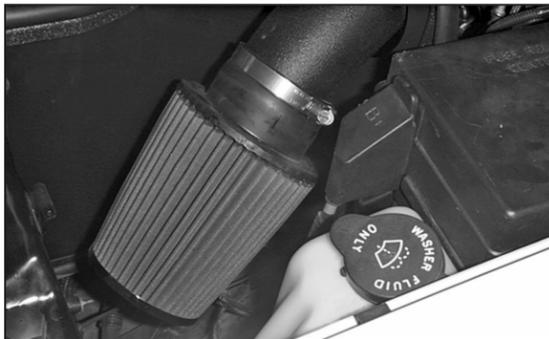
34. Install the Air Filter and tighten hose clamp.
