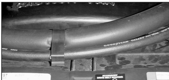
36. Secure the a/c lines to the radiator shroud with the retaining clip.
