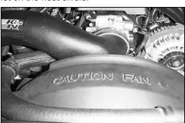
31. Due to production tolerances it may be necessary to mark the fan shroud as indicated, remove the intake tube and trim the fan shroud.
