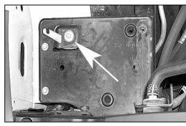
19. Loosen and remove the bolt from the airbox mounting tray.
