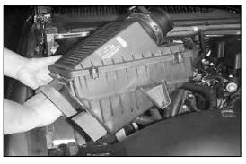
8. Pull firmly upward and remove the airbox.
