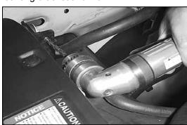
17. Using ¼" drill bit, drill out location marked in the previous step.
