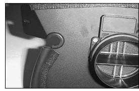
14. Install the grommet onto the heat shield.
