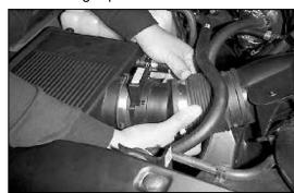
6. Detach the intake hose from the mass air sensor.
