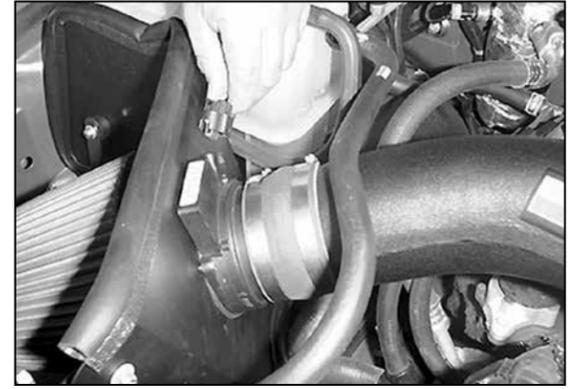
31. Reconnect the mass air sensor electrical connector.
