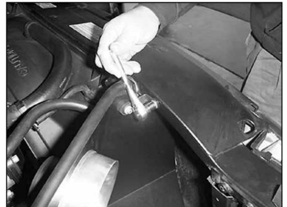
20. Secure the "L" bracket to the threaded hole in the radiator core support using the hardware provided.
