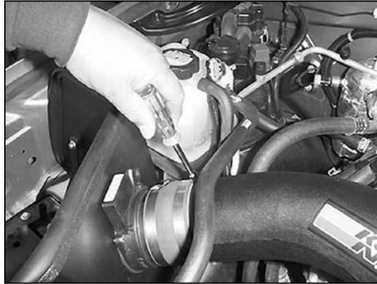
27. Tighten the hose clamp on the silicone hose at the intake tube.
