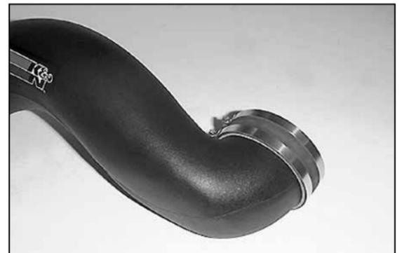
22. Install the 4"ID silicone hose onto the intake tube.
