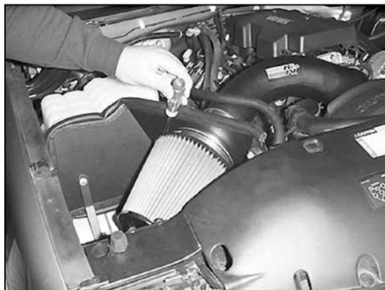
30. Install the Air filter element and secure with hose clamp.
