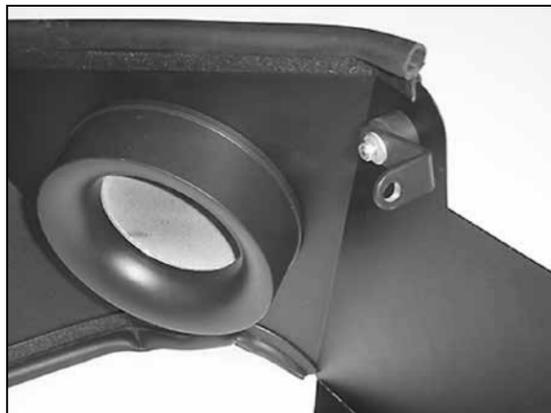
15. Attach the "L" bracket assembly to the heat shield.
