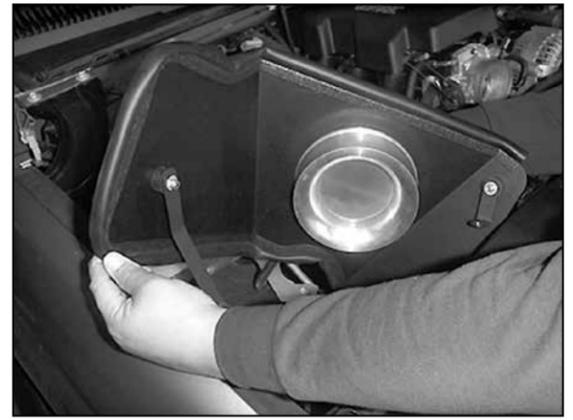
18. Install the heat shield assembly.
