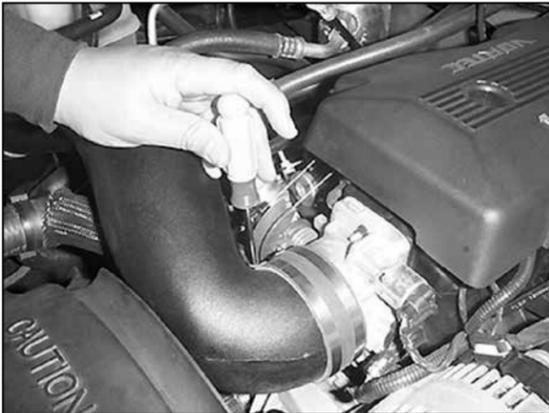
26. Align and check the intake tube for clearance, tighten the hose clamp on the silicone hose at the intake tube.
