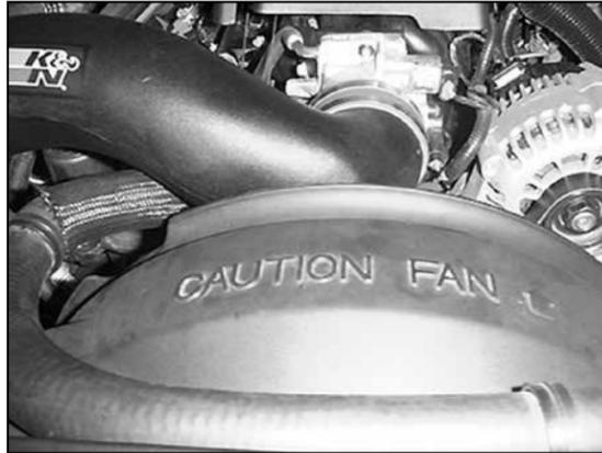
29. Due to production tolerances it may be necessary to mark the fan shroud as indicated, remove the intake tube and trim the fan shroud.
