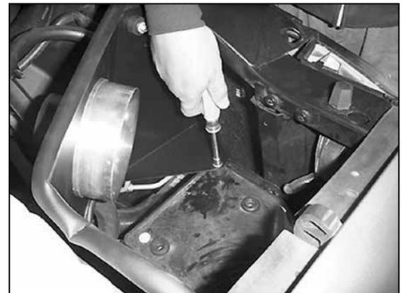
21. Secure the heat shield to the rubber mounted stud using the hardware provided.
