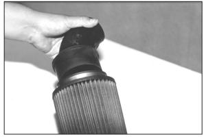
12. Assemble the tube assembly and the air filter element assembly as shown above.
