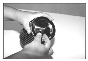
8. Install the provided rubber grommet into the air filter top as shown above.
