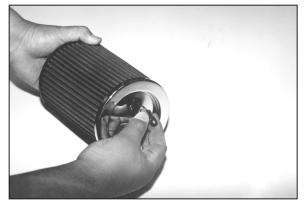
9. Insert the air temperature sensor into the rubber grommet.
