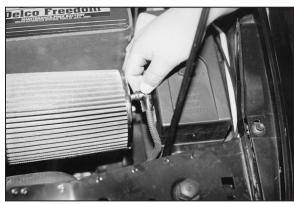
15. Re-connect the air temperature sensor electrical connection.
