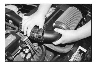
13. Install the complete assembly into the the factory intake hose.
