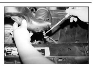
6. On 91-94 models, remove the air inlet tube and disconnect the air temperature sensor electrical connections.
