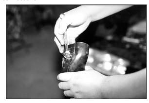
7a. On 91-94 models remove the air temperature sensor from the air inlet tube, then re-install the air inlet tube back onto the vehicle's radiator support.
