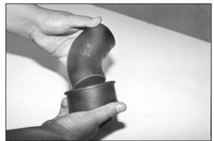
11. Install the provided velocity ring onto the K&N® intake tube as shown.
