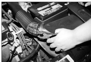
2. Loosen the hose clamp and remove the intake tube from the airbox.
