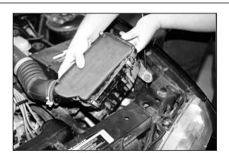
4a. On 91-94 models, remove the complete airbox assembly.
