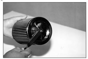
10. Assemble the provided bracket onto the air filter element using the provided hardware as shown above.
