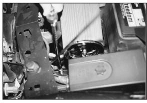
14. Secure the bracket to the existing airbox mounting hole using the provided bolt and washer. NOTE: The air temperature sensor should be located approximately in the 12 o'clock position.
