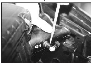
4b. On 95-96 models, disconnect the air temperature sensor electrical connection before removing the airbox assembly as shown.
