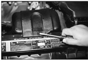
5. Remove the push clip(s) that secure the air inlet tube/resonator to the radiator support.
