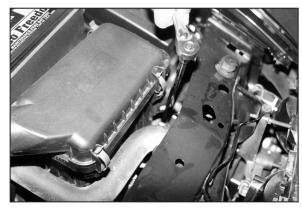
3. Using a 10mm socket, loosen and remove the three bolts that secure the airbox assembly.
