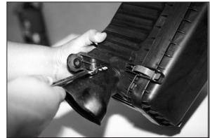
7b. On 95-96 models, remove the air temperature sensor from the air inlet tube.
