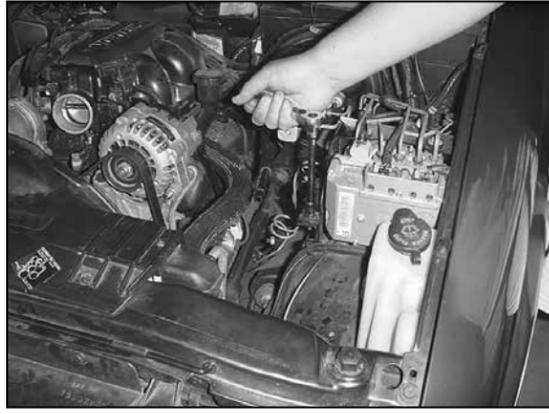
12. Using a 10mm socket, remove the bolt on the ABS bracket as shown above.
