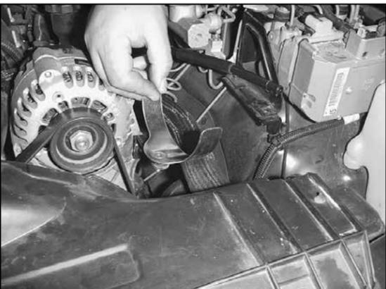
11. Install the saddle bracket assembly onto the exposed portion of the alternator pivot bolt. With the bracket positioned as shown above, tighten with the wave washer and jam nut provided.
