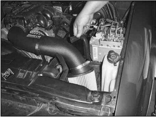
25. Install the trim seal provided onto the heat shield as shown above.
