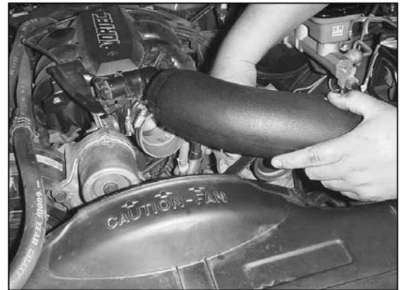
21. Install the K&N® intake tube, resting comfortably on the saddle/bracket and inserting the one end of the tube into the silicone hose. Reconnect the air temperature sensor electrical connection and insert the vent hose into the grommet hole located on the backside of the K&N tube.
