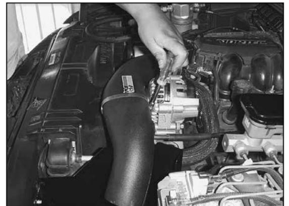
23. Install the hose clamp provided around intake tube and saddle and tighten as shown above.
