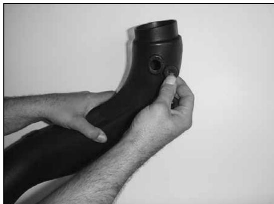
18. Install the two grommets provided into the K&N® intake tube as shown above.
