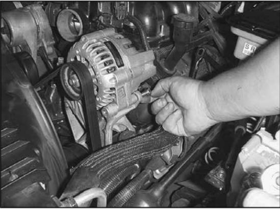
8. Remove the factory alternator pivot bolt as shown and replace it with the 10mm bolt provided, then thread into position.
