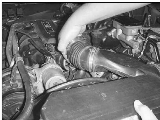
4. Remove the rubber intake hose from the throttle body and disconnect the air temperature electrical connection located on the underside of the rubber intake hose.
