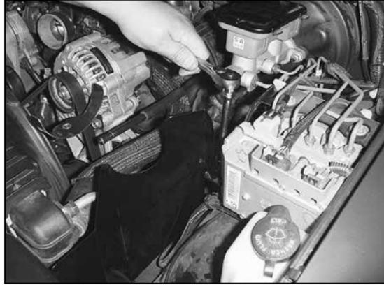
13. Install the heat shield as shown, with the factory ABS bracket bolt reinstalled.
