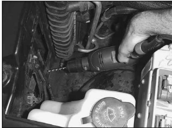
16. Using a 3/16" drill bit, drill the mark on the radiator core support.
