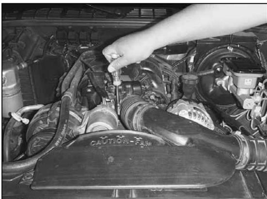
2. Loosen the hose clamp located on the rubber intake hose at the throttle body.
