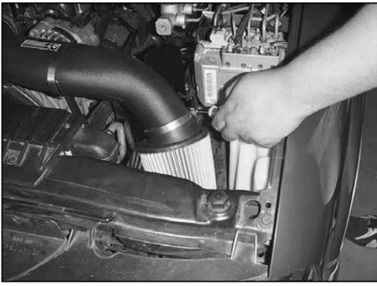
24. Install the air filter element onto the end of the intake tube. Position element for best clearance and tighten down using the provided hose clamp.
