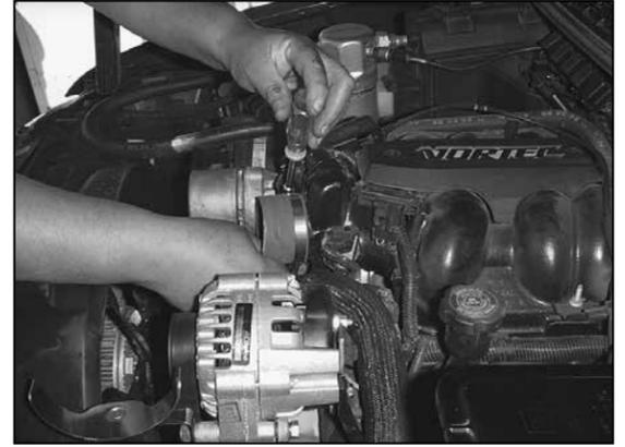
20. Install and secure the silicone hose onto the throttle body using the hose clamp provided as shown above.
