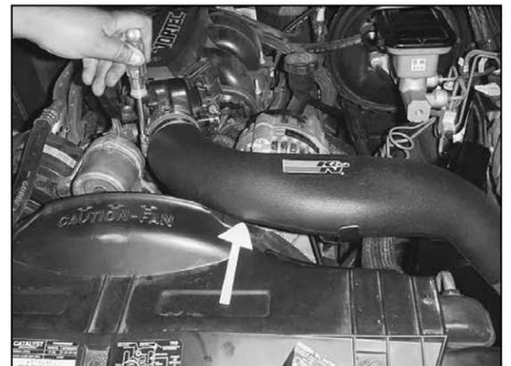
22. Tighten the silicone hose around the intake tube with the hose clamp provided.
