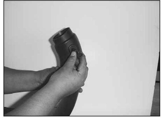
19. Remove the air temperature sensor from the factory intake hose and reinstall it into the grommet hole on the underside of the K&N® intake tube as shown above.
