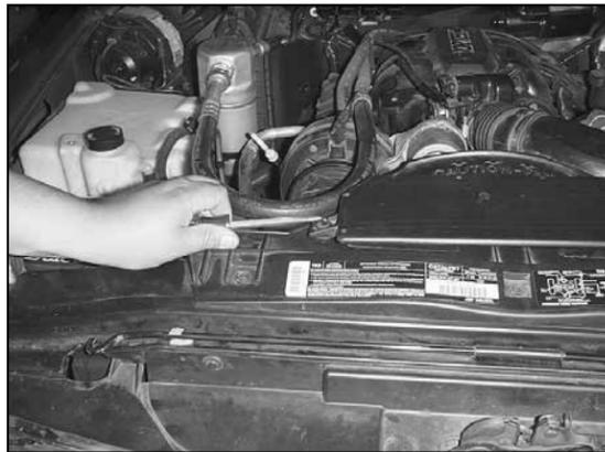
3. Using a flat blade screwdriver, release the push clip that secures the plastic resonator chamber to the radiator fan shroud.
