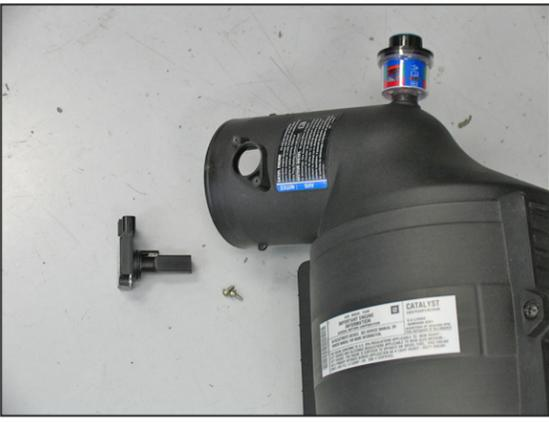
7. Using the "TORX" T20 wrench provided, remove the two bolts, which secure the mass air sensor to the air filter housing and then remove the mass air sensor.
