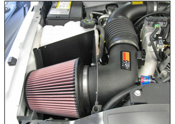
19. Install the K&N® filter onto the K&N® intake tube and secure with the provided hose clamp.
