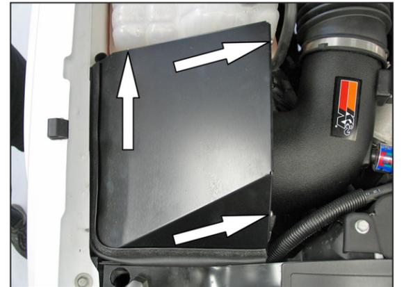
21. Install the heat shield lid onto the heat shield and secure with the three 5mm button head allen bolts provided.
