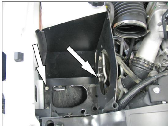
16. Install the heat shield onto the air box mounting plate and secure with the factory bolts removed in step #6.
