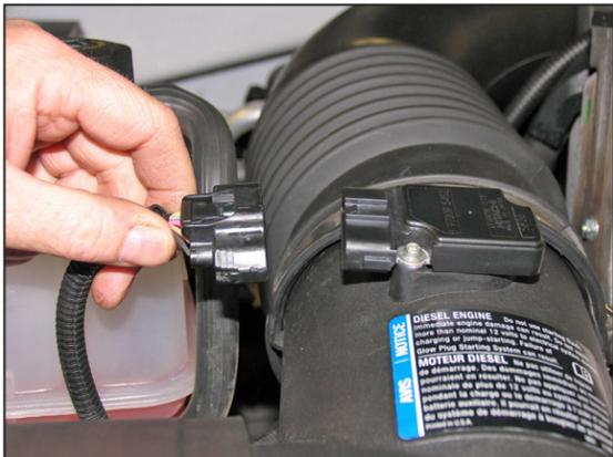
2. Depress the locking tab on the mass air sensor electrical connector, and then disconnect the electrical connection as shown.
