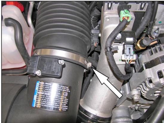
3. Loosen the hose clamps which secure the air filter housing to the stock intake tube.
