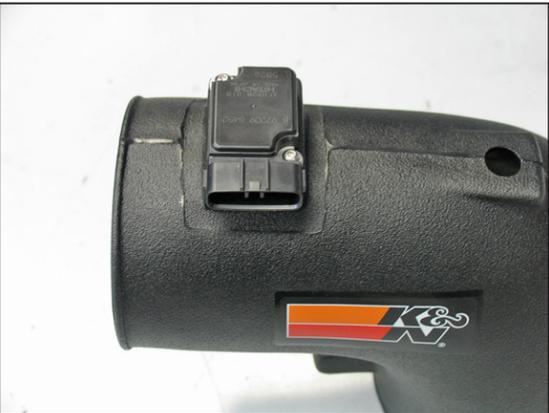
10. Install the two spacers under the mass air sensor then attach the mass air sensor to the K&N® intake tube with the provided hardware.
