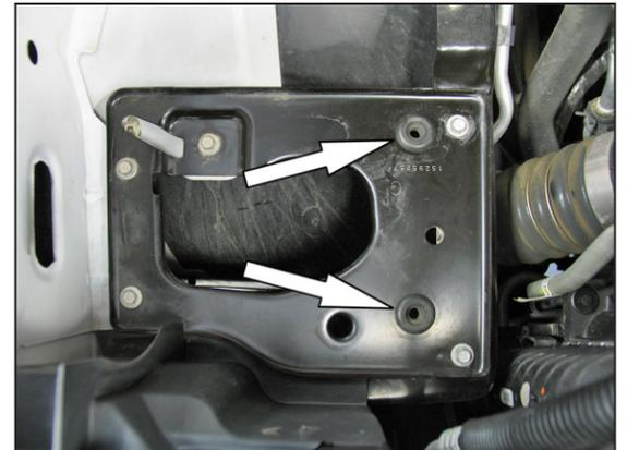
5. Remove the two mounting grommets shown from the mounting plate.
