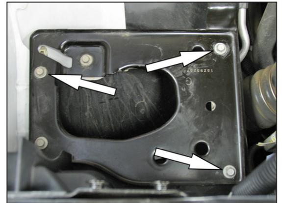
6. Remove the three bolts shown which secure the mounting plate.
