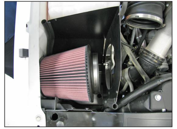
17. Set the K&N® filter into the heat shield as shown.
