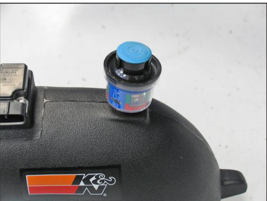
11. Install the factory grommet and filter restriction gauge into the K&N® intake tube as shown.
