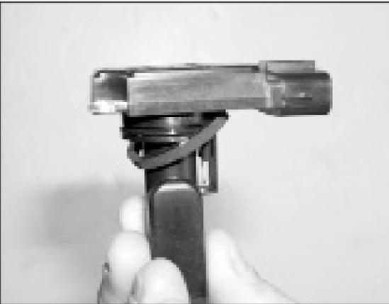
9. Install new gasket onto mass air sensor as shown with stickyside towards mass air sensor.
