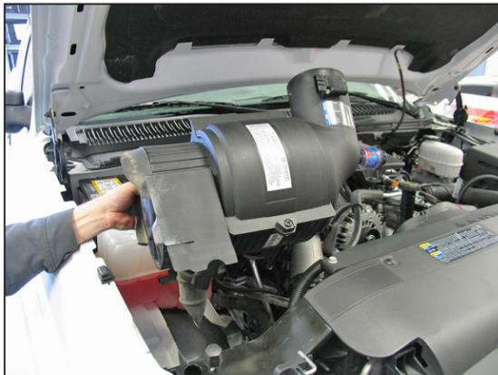
4. Lift up the air filter housing to release it from the mounting grommets, and then remove the air filter housing from the vehicle as shown.
