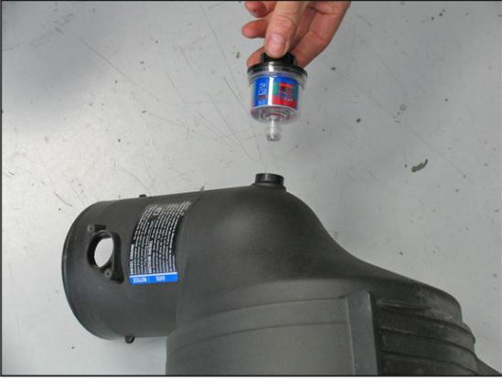
8. Remove the air filter restriction gauge and stock grommet from the air filter housing as shown.
