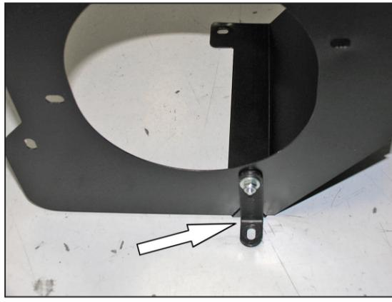
12. Install the "L" bracket (07805) onto the heat shield as shown with the provided hardware as shown.
