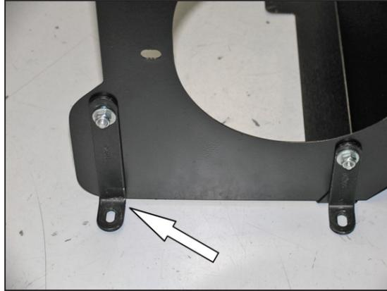
13. Install the "L" bracket (070952) onto the heat shield as shown with the provided hardware as shown.
