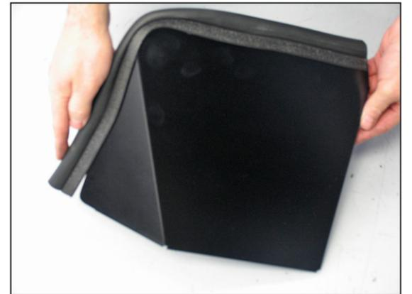
20. Install the edge trim onto the heat shield lid as shown.
