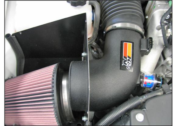
18. Install the K&N® intake tube into the heat shield and into the stock intake tube, then secure the K&N® intake tube to the heat shield with the hardware provided and hose clamp at the stock intake tube.
