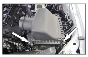
5. Release the two clips securing the upper air filter housing and then remove the upper filter housing and stock air filter.
