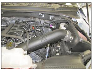
Install the K&N<sup>®</sup> intake into the coupling hose at the filter adapter and then into the hose at the throttle body, adjust the tube for best fit and then secure with the provided hose clamps.
