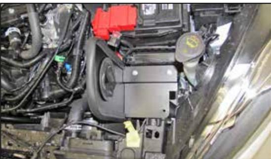
11. Install the heat shield into the vehicle so that the two mounting posts engage the air box mounting grommets.
