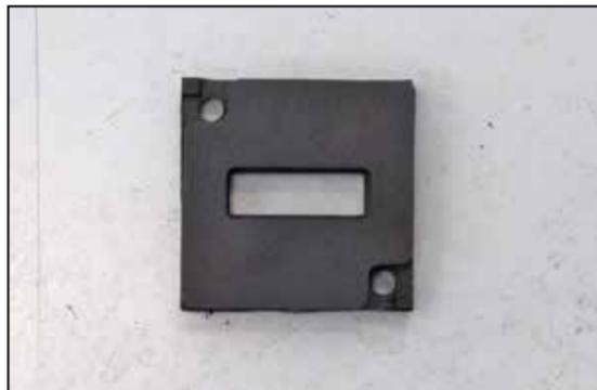
16. Install the provided gasket onto the K&N® mass air sensor adapter.
