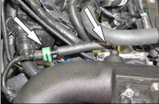
23. Install the EVAP hose assembly into the factory quick disconnect fitting and then onto the 90° fitting install into the K&N® intake tube as shown.
