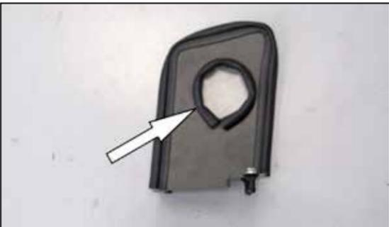
10. Install the provided "Side Bulb" edge trim around the inside of the hole in the heat shield as shown.
