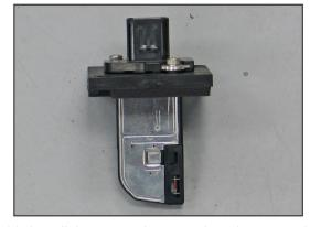
20. Install the mass air sensor into the mass air sensor adapter and secure with the provided hardware.
