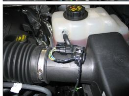
2. On vehicles equipped with a mass air sensor, release the red locking tab and then disconnect the mass air sensor electrical connection. On vehicles equipped with a pressure sensor, disconnect the electrical connection and then unhook the wiring harness from the stud.
