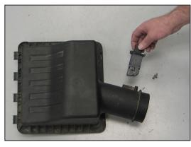
19. If the vehicle is equipped with a mass air sensor, remove the two bolts securing the mass air sensor into the factory air box and then remove the sensor from the air box.
