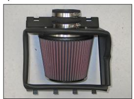
12. Install the provided silicone hump hose (08699) onto the filter adapter and secure with the provided hose clamp.
