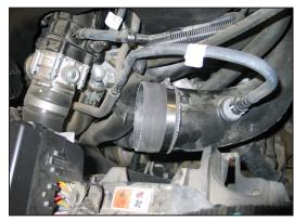
15. Install the provided silicone hose (08761) onto the driver's side turbo inlet tube and secure with the provided hose clamp.
