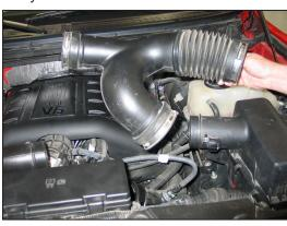
5. Remove the factory intake tube as shown. NOTE: DO NOT remove the air diverters from the factory turbo inlet tubes.
