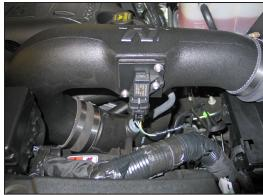
27. Reconnect the mass air sensor or pressure sensor electrical connection. Secure the sensor wiring harness to the main harness with the provided tie wrap.
