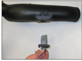
21. Install the mass air sensor assembly into the  $K\&N^{\otimes}$  intake tube and secure with the provided hardware.
