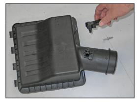
22. If the vehicle is equipped with a pressure sensor, remove the bolt securing the pressure sensor into the factory air box, and then remove the sensor from the air box.
