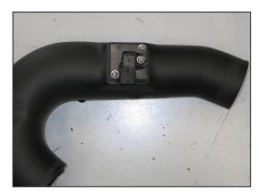
24. Install the pressure sensor assembly into the K&N® intake tube and secure with the provided hardware.
