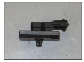
23. Install the pressure sensor into the pressure sensor adapter and secure with the provided hardware.
