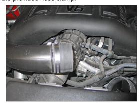
16. Install the provided silicone hose (08711) onto the passenger side turbo inlet tube and secure with the provided hose clamp.
