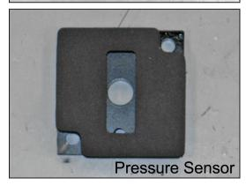
18. With vehicles equipped with a mass air sensor, install the provided gasket onto the mass air sensor adapter. On vehicles equipped with a pressure sensor, install the provided gasket onto the pressure sensor adapter as shown.
