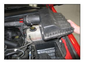
6. Release the three locking tabs and then lift up and remove the upper air box from the vehicle.
