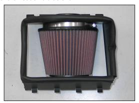
11. Install the K&N® air filter onto the filter adapter and secure with the provided hose clamp.
