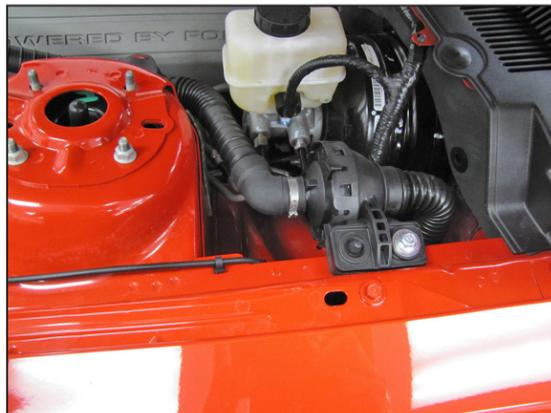
4. Cut the clamp securing the sound tube to the sound drum and then disconnect the sound tube from the drum.
