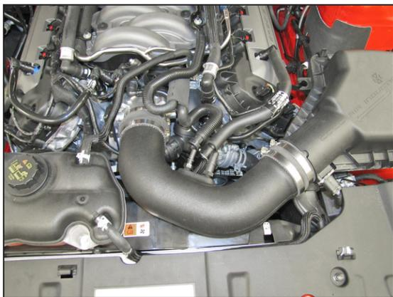
14. Install the K&N® intake tube into the hose at the air box and then into the hose at the throttle body. Adjust the tube for proper fitment and then secure with the provided hose clamps.
