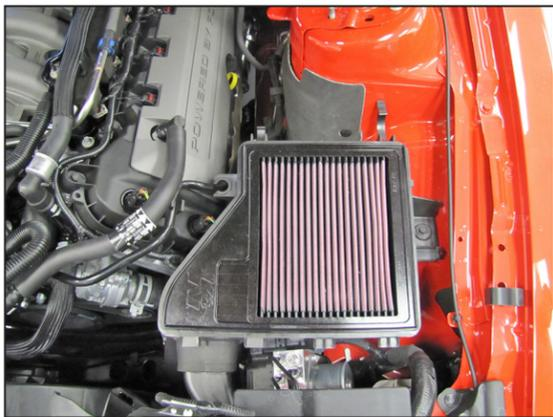
10. Remove the factory air filter and replace with the provided K&N® air filter, then reinstall the air box lid.
