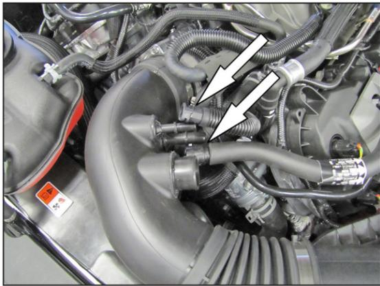
7. On vehicle equipped with an EVAP vent line, disconnect the EVAP vent line from the factory intake tube. Disconnect the crank case vent hose from the factory intake tube.
