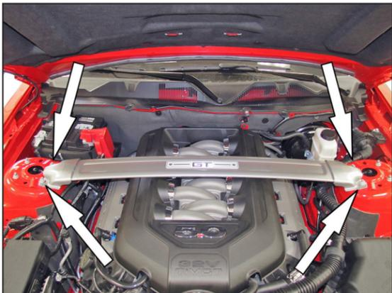
2. Remove the four nuts securing the strut bar and then remove the strut bar from the vehicle.
