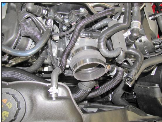
11. Install the provided coupling hose (08699) onto the throttle body and secure with the provided hose clamp.
