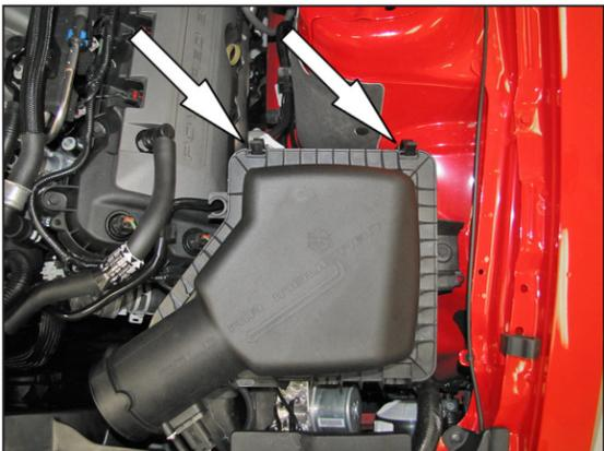
9. Release the air box retaining clips and lift off the upper air box.
