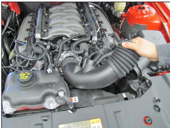
8. Loosen the hose clamps securing the factory intake tube and remove the intake tube from the vehicle.
