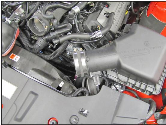
12. Install the provided coupling hose (08536) onto the air box outlet and secure with the provided hose clamp.
