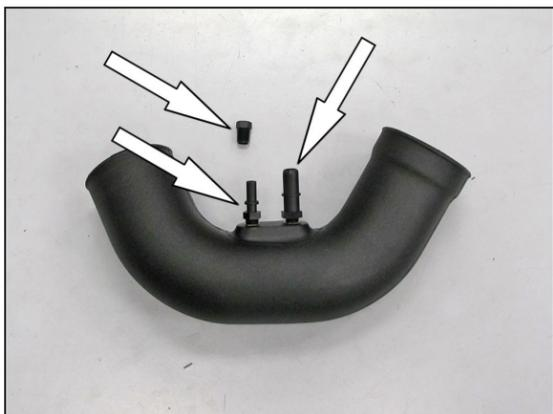
13. Install the provided quick connect fittings into the K&N intake tube as shown.
