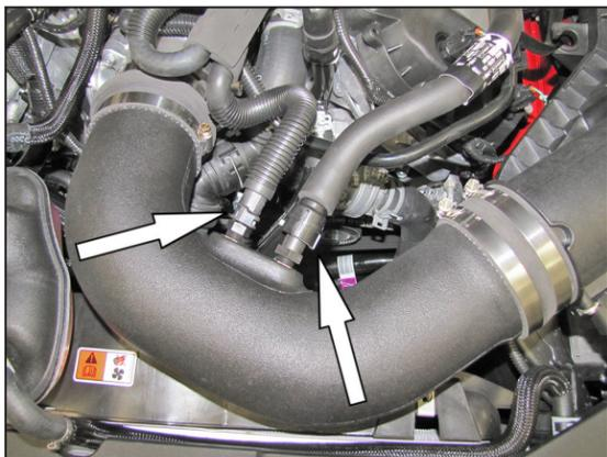
15. Connect the crank case vent hose and EVAP vent hose if equipped to the quick connect fittings as shown.
