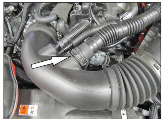
5. Release the spring clamp securing the sound tube to the intake tube and then disconnect the sound tube from the intake tube. Remove the sound tube from the vehicle.
