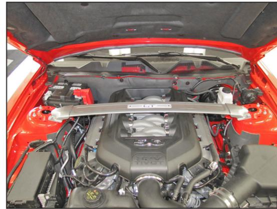
17. Reinstall the strut tower brace and secure with the factory nuts.
