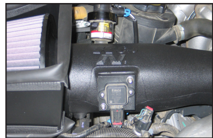
26. Reconnect the mass air sensor electrical connection.
