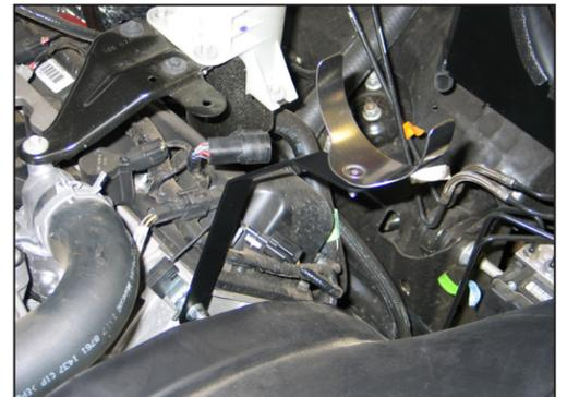
22. Install the tube mounting bracket assembly onto the stud protruding from the cylinder head. Secure with the provided hardware.
