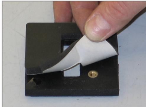
16. Install the mass air sensor gasket onto the mass air sensor adapter as shown.
