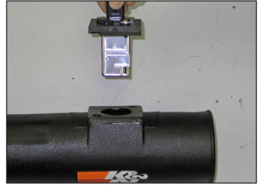
18. Install the mass air sensor assembly into the K&N® intake tube and secure with the provided hardware as shown.
