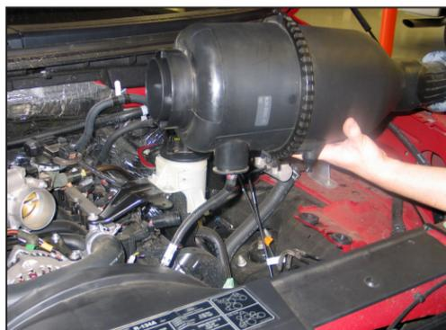
5. Pull up firmly on the air box, removing it from the mounting grommets.
