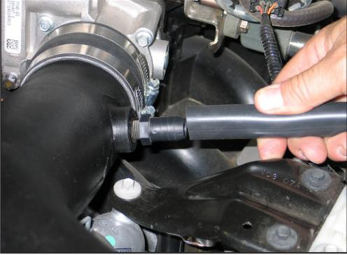
24. Connect the provided crank case vent hose onto the fitting on the valve cover and the vent fitting on the K&N® intake tube.
