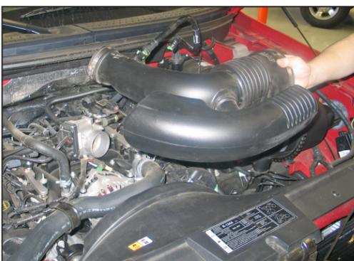
3. Loosen the stock intake tube hose clamps and remove the intake tube assembly from the vehicle.
