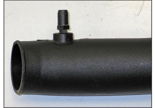
19. Install the 1/4" NPT fitting into the K&N® intake tube as shown.
