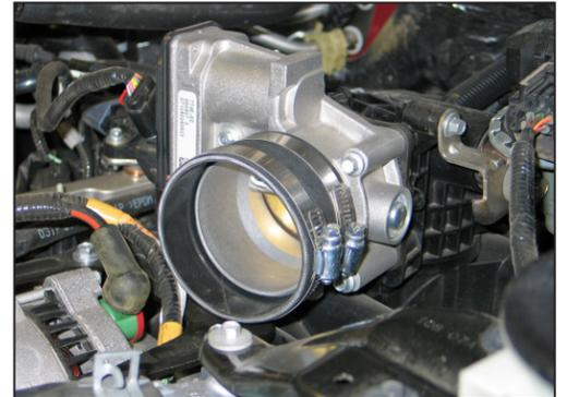
20. Install silicone hose (#08690) onto the throttle body and secure with the provided hose clamp.
