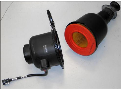
11. Release the factory air box clam shell clamp, then separate the mass air sensor housing from the factory air box.
