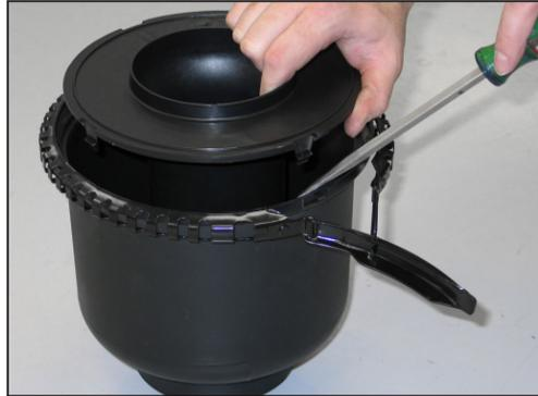
14. Using a flat blade screw driver; push in and release the four clips that secure the mass air sensor retaining plate.
