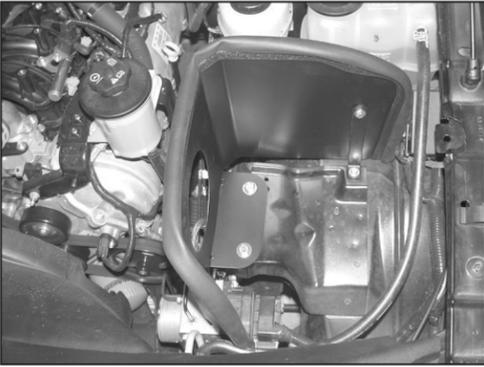
10. Install the heat shield and secure with the provided hardware as shown.
