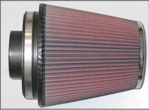
25. Install the air filter adapter into the K&N® air filter and secure the assembly with the provided hose clamp.
